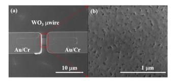
Fig. 3 Low-magnification scanning electron microscope image of the WO<sub>3</sub> microwires fabricated at 600 °C and (b) enlarged image of the red-highlighted area in (a).
