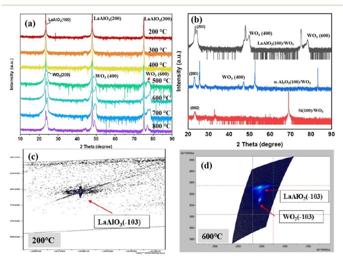
Fig. 2 X-ray diffraction patterns of the  $WO_3$  thin films deposited (a) at different temperatures on LaAlO $_3$  (100) substrates and (b) on different substrates at 600 °C. Reciprocal space maps of the  $WO_3$  thin films deposited on LaAlO $_3$  (100) substrates at (c) 200 °C and (d) 600 °C.
