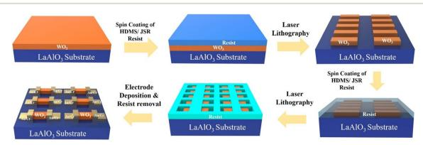
Fig. 1 Schematic of the preparation steps of the WO<sub>3</sub> microwire-based gas sensor.
