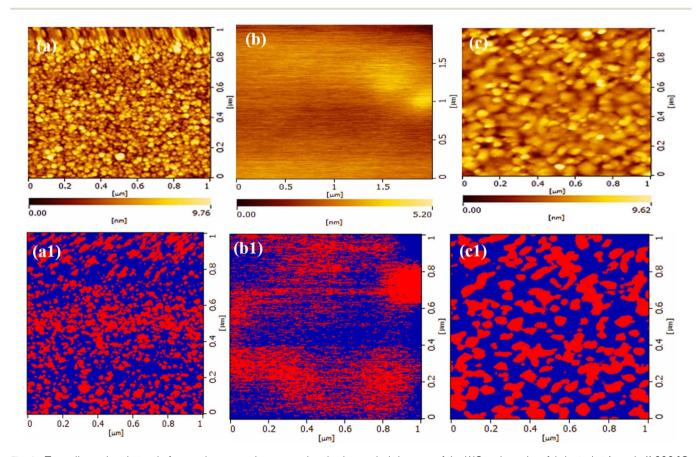
Fig. 4 Two-dimensional atomic force microscope images and grain size analysis images of the WO<sub>3</sub> microwires fabricated at (a and a1) 200 °C; (b and b1) 400 °C; and (c and c1) 600 °C.
