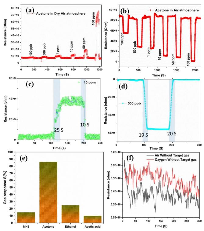
Fig. 6 Gas response and recovery plots of the a- $WO_3$  nanowire in (a and c) dry air and (b and d) ambient air, respectively. (e) Selectivity of gas sensor towards different gas molecules, (f) resistance of the gas sensor measured in dry and ambient air without target gas.
