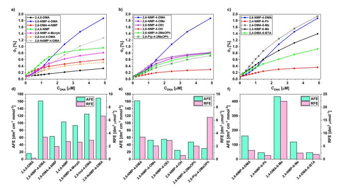
(a-c) Dependence of the effective fluorescence quantum yield ( $\Phi_{f_i}$  in percents) on the concentration of plasmid DNA. (d-f) Absolute (AFE) and relative fluorescence enhancements (RFE) of the synthesized pyrylium derivatives.
