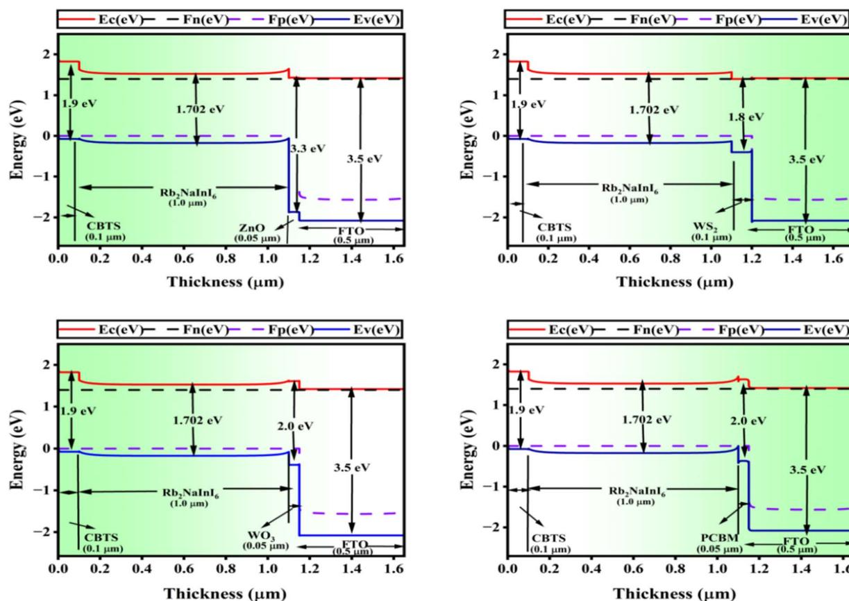
Fig. 9 Band diagram illustrating  $\text{Rb}_2\text{NaNiI}_6$ . (a) ZnO, (b)  $\text{WS}_2$ , (c)  $\text{WO}_3$ , and (d) PCBM are the first four.
