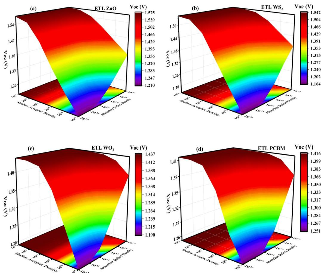
Fig. 14 Three-dimensional surface plot of both open-circuit voltage ( $V_{oc}$ ) being a function of shallow acceptor density ( $N_A$ ) in addition to absorber defect density ( $N_D$ ) for perovskite solar cells (PSCs) utilizing (a) ZnO, (b)  $\text{WS}_2$ , (c)  $\text{WO}_3$ , and (d) PCBM electron transport layers (ETLs).
