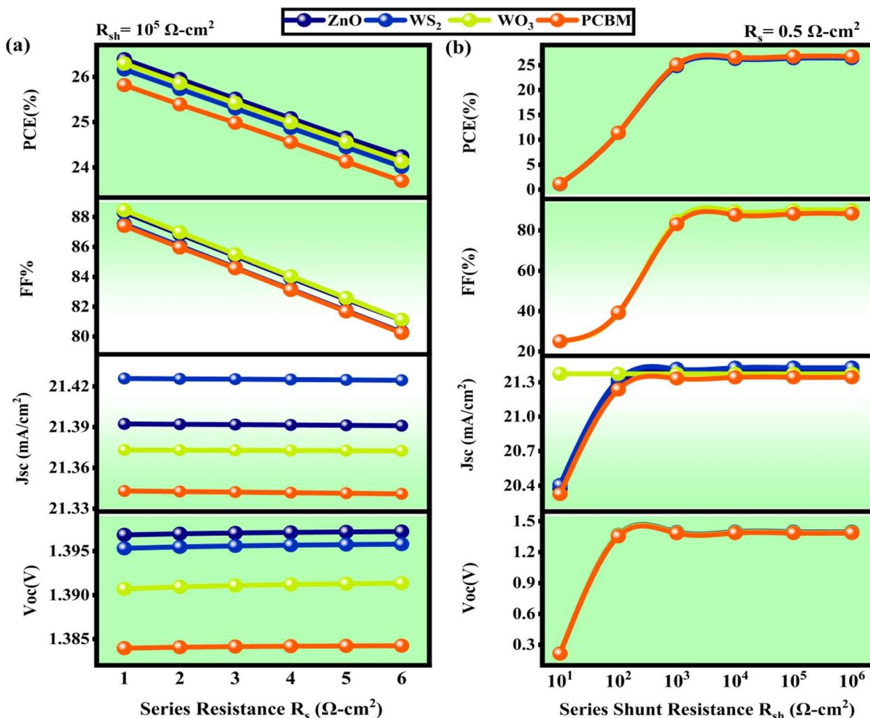
Fig. 19 Effectiveness variations in (a) Shunt resistance ( $R_{sh}$ ) and (b) series resistance ( $R_s$ ) both on  $V_{oc}$  (V),  $J_{sc}$  ( $\text{mA cm}^{-2}$ ), FF (%), and PCE (%).
