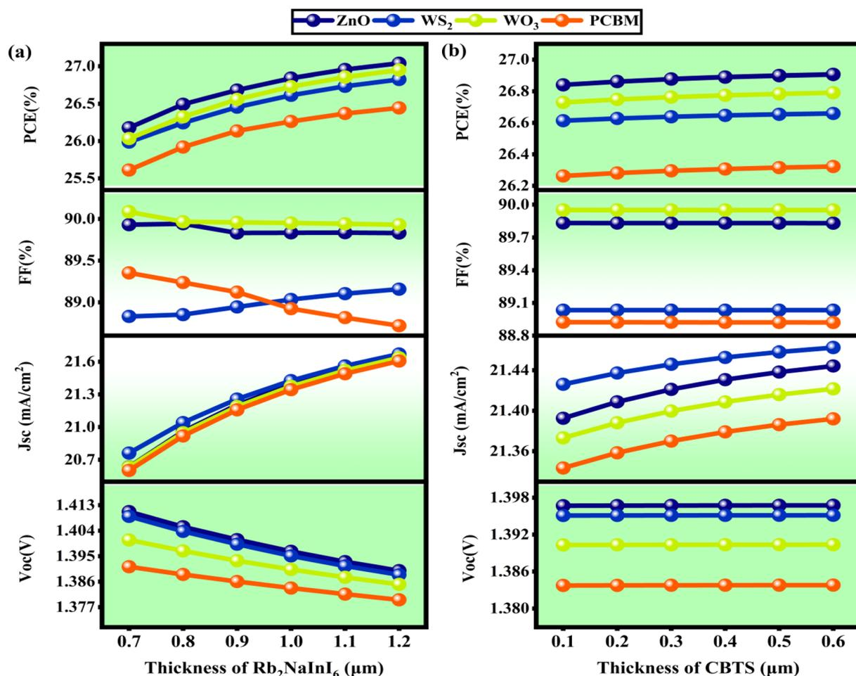
Fig. 18 The influence of modifications in (a) Rb<sub>2</sub>NaInI<sub>6</sub> and (b) CBTS thickness demonstrates the effects on  $V_{oc}$  (V),  $J_{sc}$  (mA cm<sup>-2</sup>), FF (%), and PCE (%).
