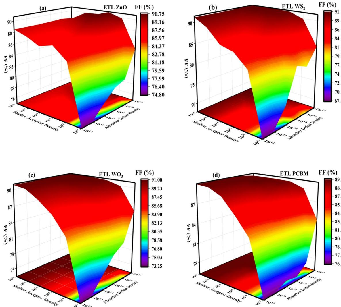
Fig. 16 Three-dimensional surface plot of both fill factor (FF) being a function of shallow acceptor density ( $N_A$ ) in addition to absorber defect density ( $N_D$ ) for perovskite solar cells (PSCs) utilizing (a) ZnO, (b)  $WS_2$ , (c)  $WO_3$ , and (d) PCBM electron transport layers (ETLs).
