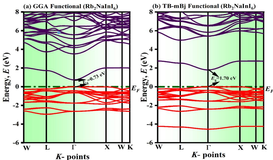
Fig. 5 Electronic band structure of  $\text{Rb}_2\text{NaInI}_6$ .
