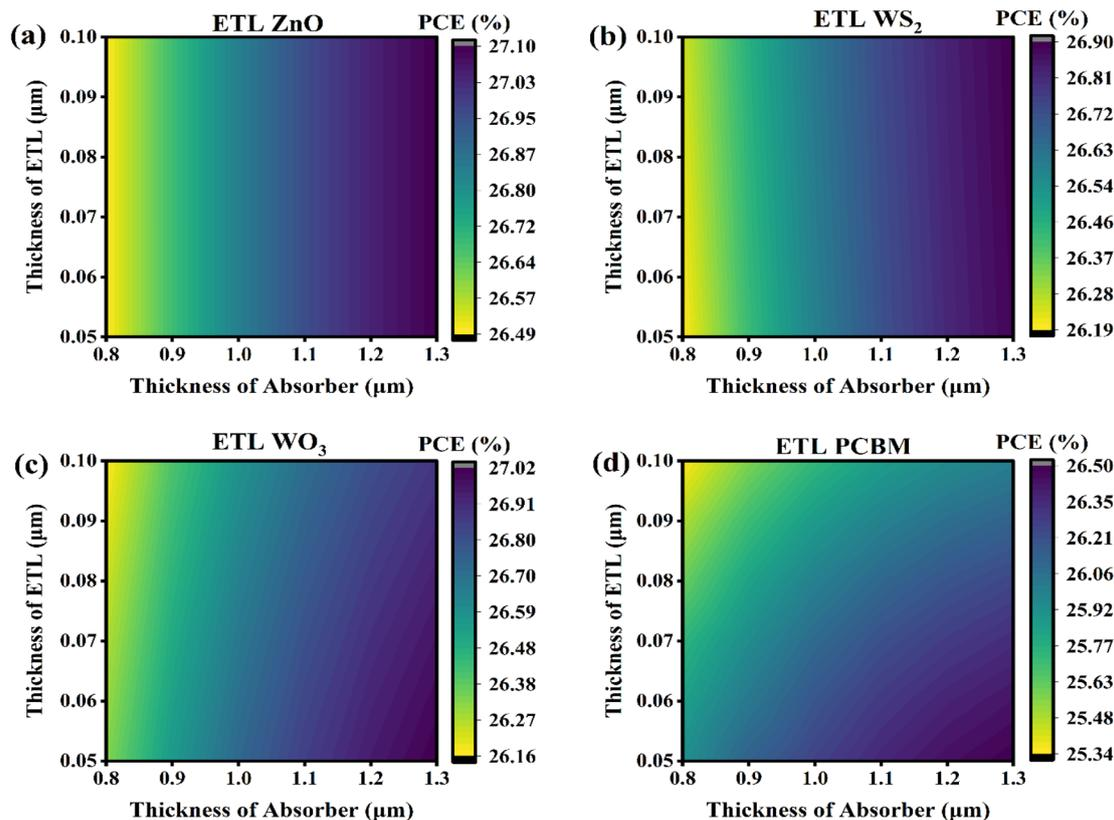
Fig. 13 Contour mapping of PCE (%) when ETL is (a) ZnO, (b) WS<sub>2</sub>, (c) WO<sub>3</sub>, (d) PCBM.
