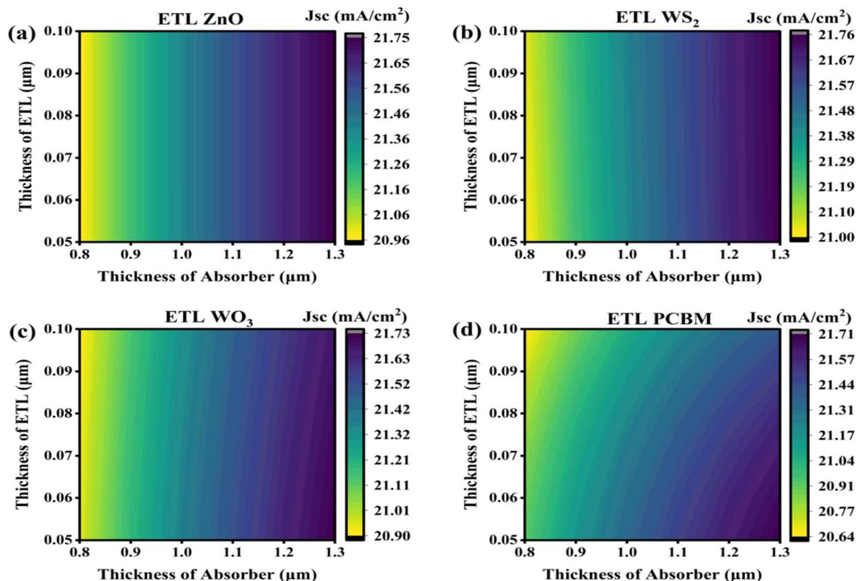
Fig. 11 Contour modeling of the  $J_{sc}$  ( $\text{mA cm}^{-2}$ ) with the HTL-like (a) ZnO, (b) WS<sub>2</sub>, (c) WO<sub>3</sub>, (d) PCBM.
