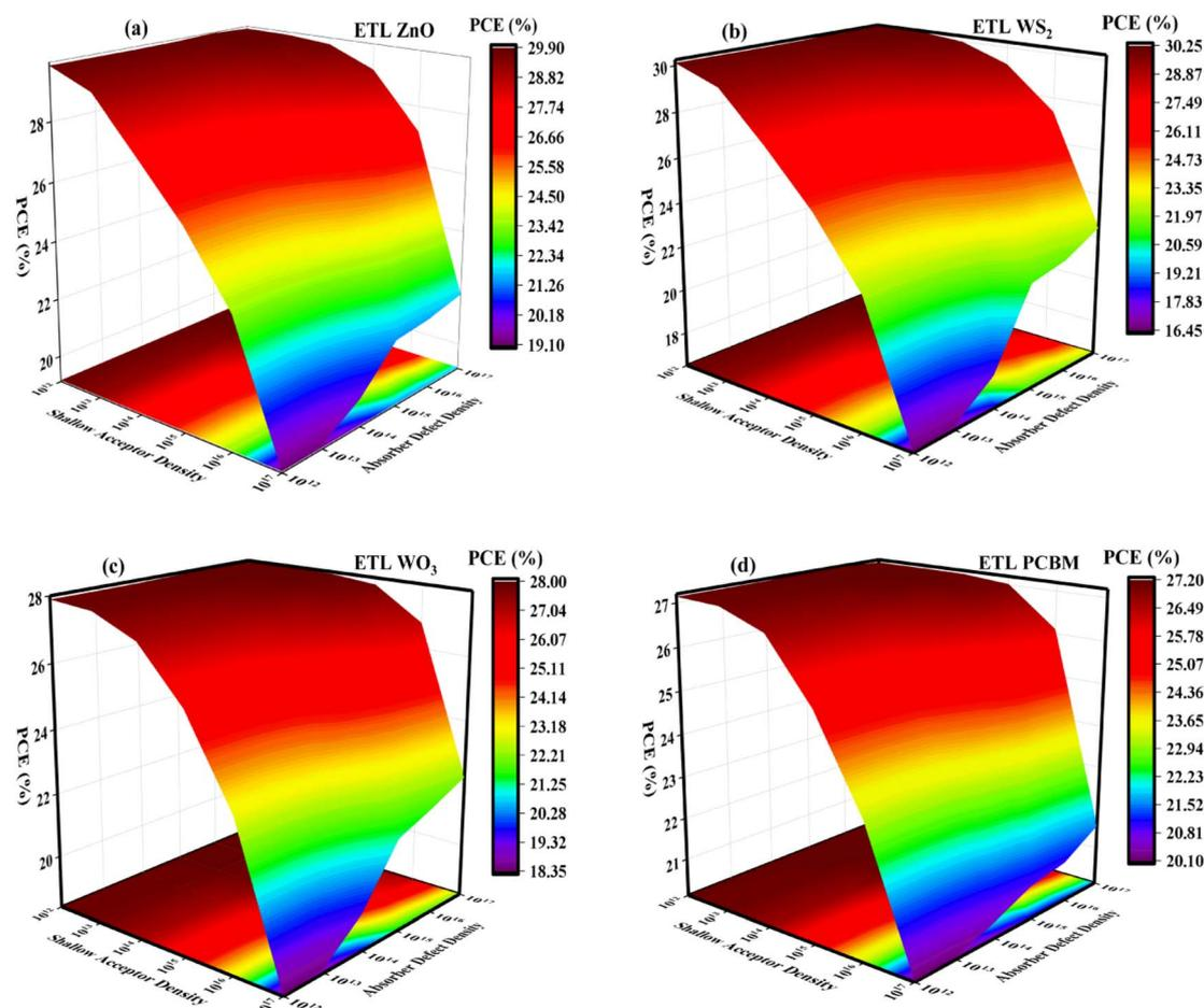
Fig. 17 Three-dimensional surface plot of both power conversion efficiency being a function of shallow acceptor density ( $N_A$ ) in addition to absorber defect density ( $N_D$ ) for perovskite solar cells (PSCs) utilizing (a) ZnO, (b)  $\text{WS}_2$ , (c)  $\text{WO}_3$ , and (d) PCBM electron transport layers (ETLs).
