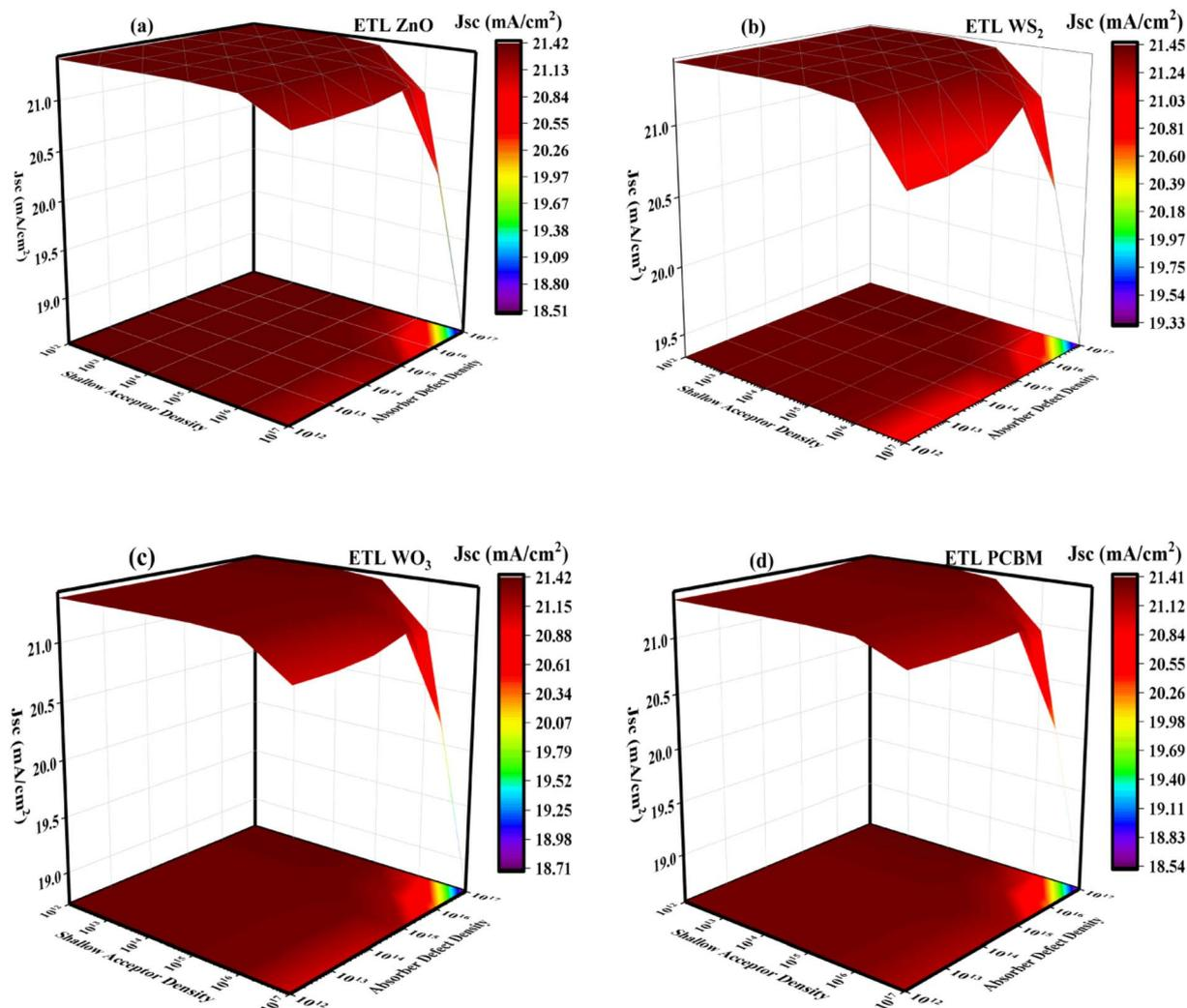
Fig. 15 Three-dimensional surface plot of both short-circuits voltage ( $J_{sc}$ ) being a function of shallow acceptor density ( $N_A$ ) in addition to absorber defect density ( $N_D$ ) for perovskite solar cells (PSCs) utilizing (a) ZnO, (b)  $WS_2$ , (c)  $WO_3$ , and (d) PCBM electron transport layers (ETLs).
