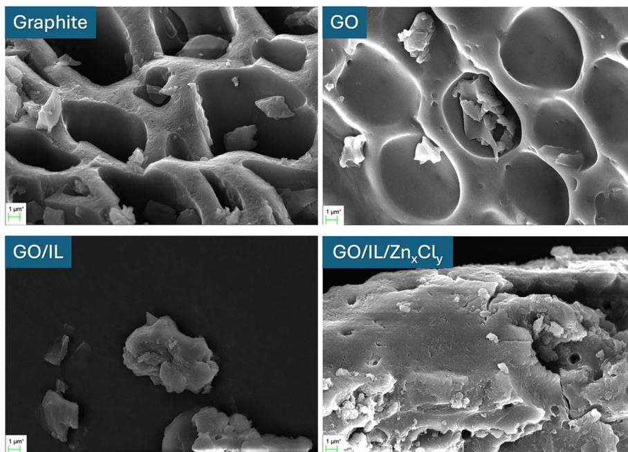
Fig. 5 FESEM images of graphite, GO, GO/IL, and GO/IL/Zn<sub>x</sub>Cl<sub>y</sub>.
