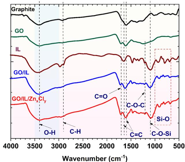
Fig. 1 FT-IR spectra of graphite, GO, IL, GO/IL, and GO/IL/Zn<sub>x</sub>Cl<sub>y</sub>.
