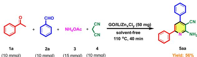
Scheme 5 Examination of scale-up in the 5aa production process employing the GO/IL/Zn<sub>x</sub>Cl<sub>y</sub> catalyst.
