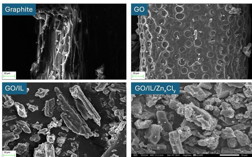
Fig. 4 SEM images of graphite, GO, GO/IL, and GO/IL/Zn<sub>x</sub>Cl<sub>y</sub>.
