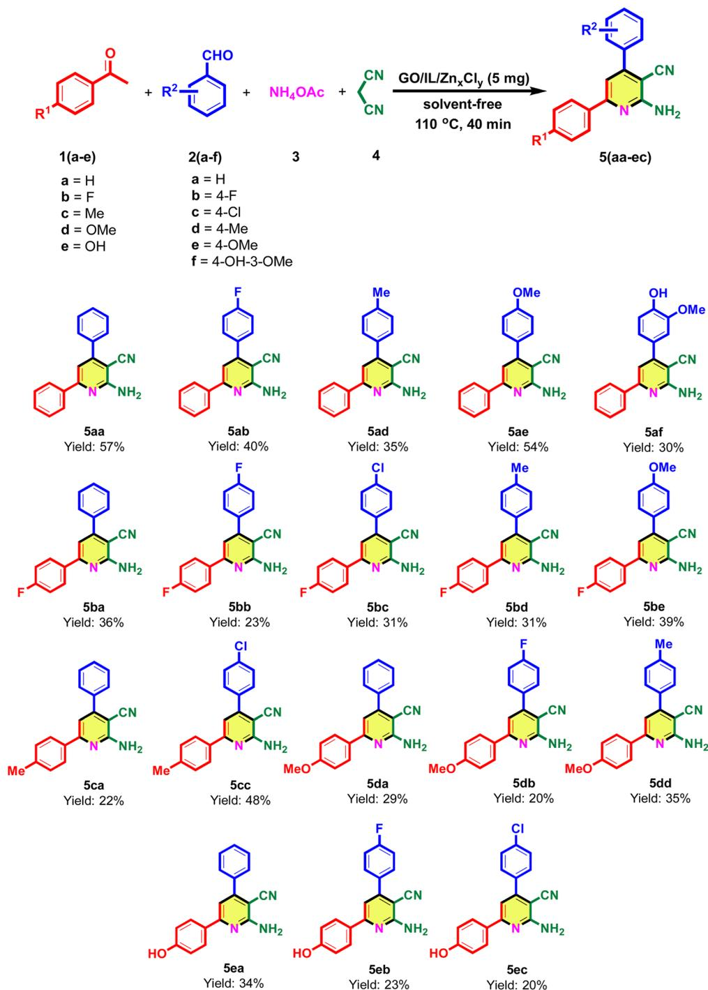
**Scheme 3** Scope of 2-amino-3-cyanopyridine derivatives.<sup>a</sup> Reaction conditions: arylaldehyde (1.0 mmol), acetophenones (1.0 mmol), ammonium acetate (1.5 mmol), malononitrile (1.0 mmol), GO/IL/Zn<sub>x</sub>Cl<sub>y</sub> (5 mg), solvent-free, 110 °C, 40 min. Isolated yield by crystallization in ethanol (15–20 mL).
