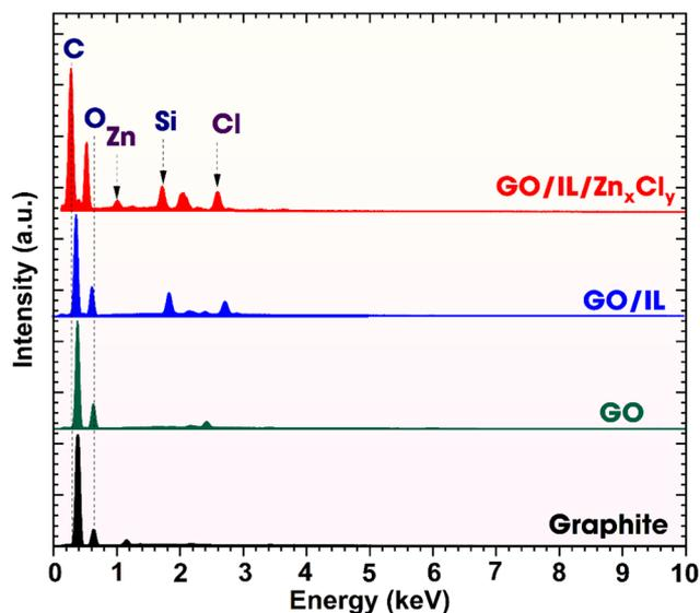
Fig. 7 EDS spectroscopy of graphite, GO, GO/IL, and GO/IL/Zn<sub>x</sub>Cl<sub>y</sub>.
