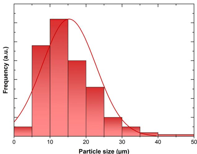
Fig. 6 Particle size distributions of GO/IL/Zn<sub>x</sub>Cl<sub>y</sub>.
