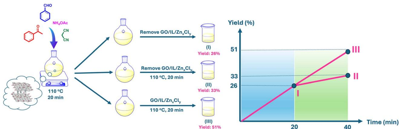
Scheme 6 Leaching test procedure: (I) reaction stopped; (II) reaction without GO/IL/Zn<sub>x</sub>Cl<sub>y</sub>; (III) continuous reaction with GO/IL/Zn<sub>x</sub>Cl<sub>y</sub>.
