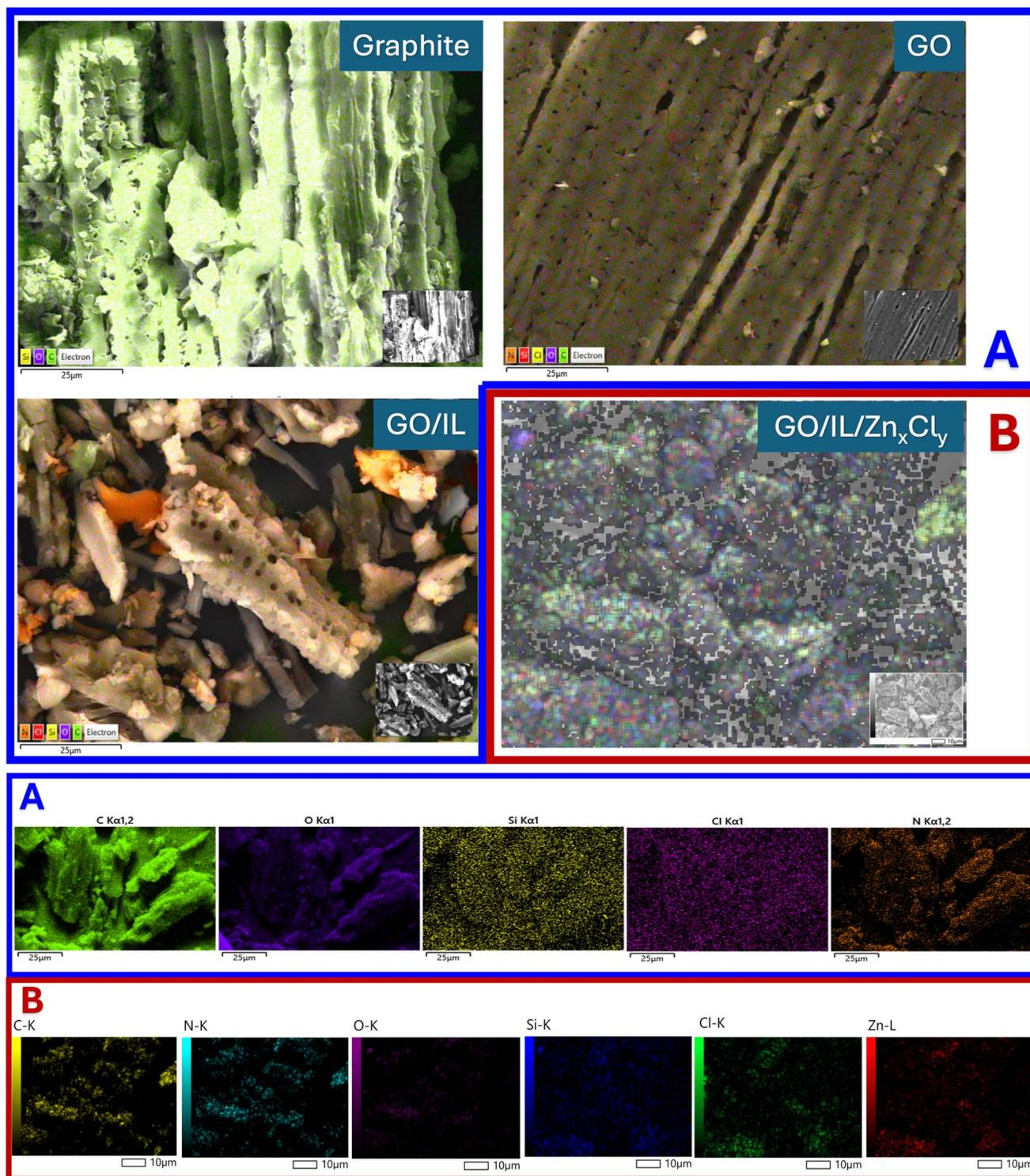
Fig. 8 EDS mapping of graphite, GO, GO/IL, and GO/IL/Zn<sub>x</sub>Cl<sub>y</sub>.
