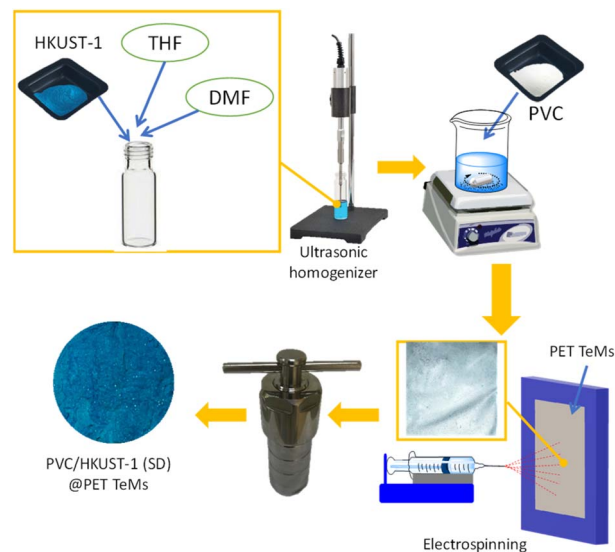
Fig. 1 Schematic of the preparation of PVC/HKUST-1 (SD)@PET TeMs.
