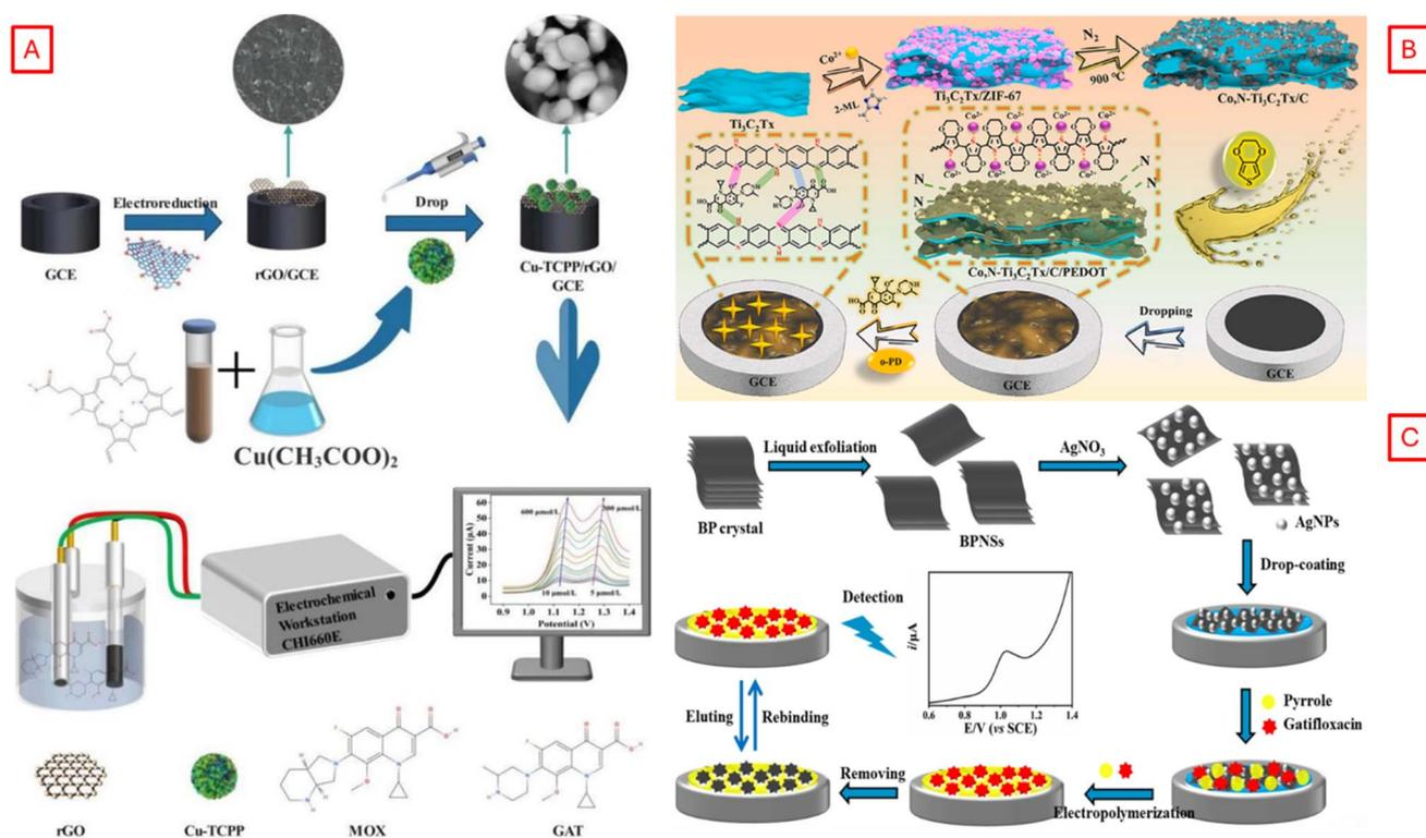
Fig. 5 Electrochemical detection of gatifloxacin based on (A) Cu-TCPP/rGO;<sup>122</sup> (B) defect-rich Co, N-doped Ti<sub>3</sub>C<sub>2</sub>T<sub>x</sub>/Cpoly(3,4-ethylenedioxy thiophene);<sup>123</sup> (C) BPNS-AgNP/GCE based molecularly imprinted sensors.<sup>124</sup>
