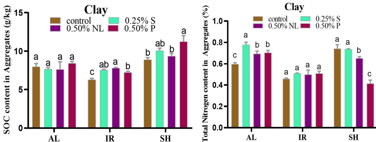
Fig. 5 Distribution of SOC and TN content in the <0.053 mm aggregate fraction after the application of S, NL and P FA to AL, IR and SH soils. Standard errors of the mean ( $n = 4$ ) are shown by error bars. At the 5% level of significance, the least significant difference (LSD 0.05) is presented. The letters above each bar (a, b, and c) indicate a substantial difference between the treatments.
