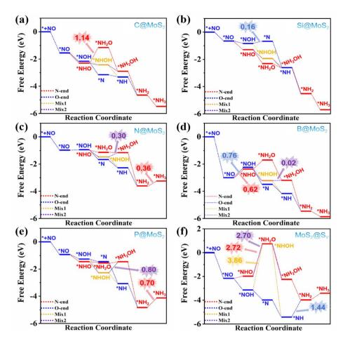
Fig. 7 Free energy diagrams of eNORR to NH<sub>3</sub> over five NM@MoS<sub>2</sub> catalysts and one MoS<sub>2</sub>@V<sub>S</sub> catalysts; (a) C@MoS<sub>2</sub>; (b) Si@MoS<sub>2</sub>; (c) N@MoS<sub>2</sub>; (d) B@MoS<sub>2</sub>; (e) P@MoS<sub>2</sub>; (f) MoS<sub>2</sub>@S<sub>v</sub>.
