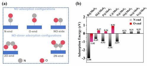
Fig. 3 (a) Possible NO adsorption configurations both high and low NO concentration; (b) NO adsorption energy on NM@MoS2 catalyst.
