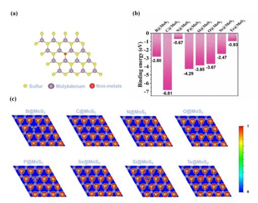
Fig. 1 (a) The modeled structure of NM@MoS<sub>2</sub> catalysts (top); (b) binding energies of NM@MoS<sub>2</sub> catalysts; (c) ELF diagram of NM@MoS<sub>2</sub> catalysts.
