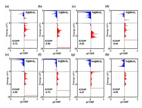
Fig. 2 COHP describes the interaction between the NM and Mo in the NM-Mo bond, while ICOHP represents the strength of this bond (the dashed line corresponds to the Fermi level). (a)  $B@MoS_2$ ; (b)  $C@MoS_2$ ; (c)  $N@MoS_2$ ; (d)  $O@MoS_2$ ; (e)  $P@MoS_2$ ; (f)  $Si@MoS_2$ ; (g)  $Se@MoS_2$ ; (h)  $Te@MoS_2$ .
