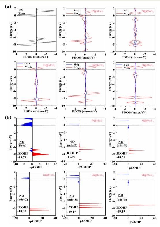
Fig. 5 (a) PDOS diagram of NO adsorption on NM@MoS $_2$  catalyst; (b) the COHP diagram of NO before and after adsorption. The left side corresponds to the antibonding orbital of the N=O bond and the right side to the bonding orbital. The labelled value of ICOHP indicates the strength of the N=O bond in the N=O bond.
