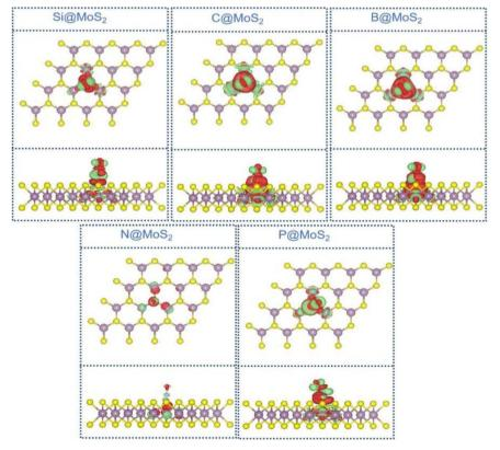
Fig. 4 CDD diagram of NO adsorption on NM@MoS<sub>2</sub> catalyst. The isosurface value is set to 0.002 e  $Å^{-3}$ .
