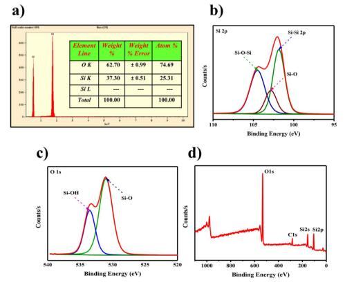
Fig. 4 SiQDs. (a) Energy Dispersive X-ray Analysis (EDAX) for elemental composition; (b-d) X-ray Photoelectron Spectroscopy (XPS) spectra illustrating surface chemical states and bonding environment.
