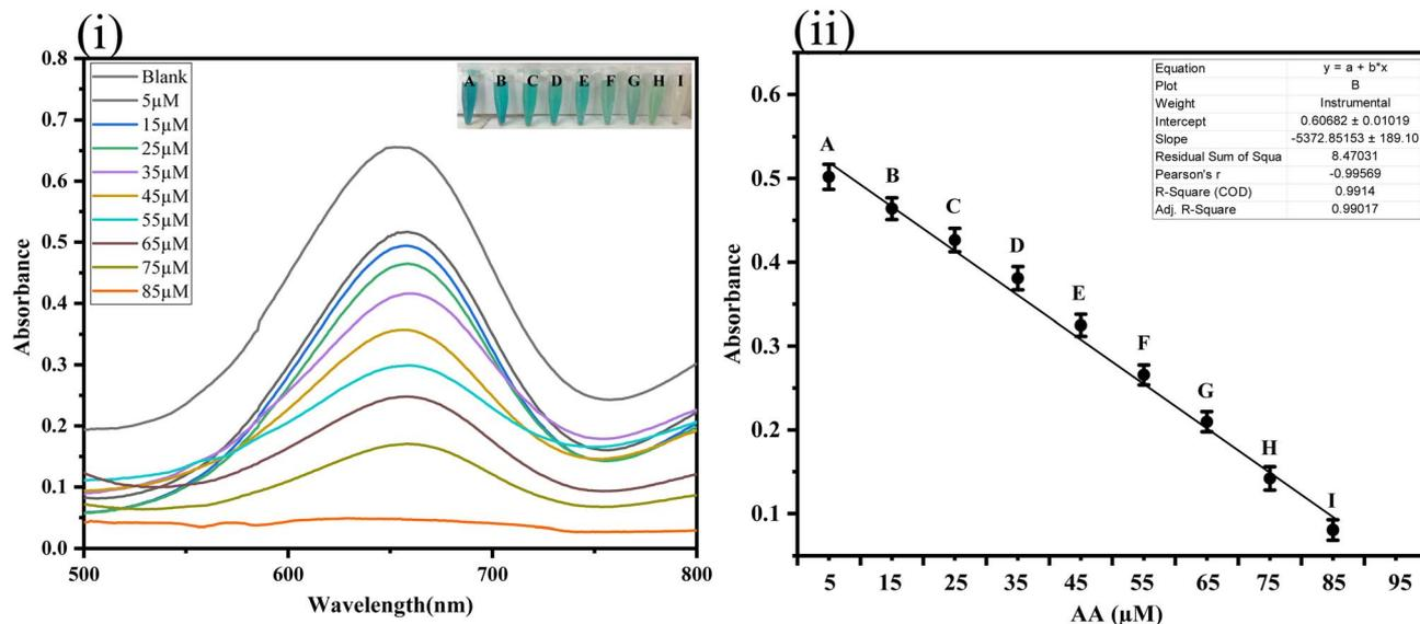
Fig. 6 Analytical performance of the sensing platform represented by the corresponding inset Eppendorf tubes. (i) UV-visible results of the analyte concentrations in the range of 5–85  $\mu\text{M}$  with a linear change in absorbance. (ii) Quantitative relationship between the concentration of ascorbic acid and absorbance ( $n = 3$ ).
