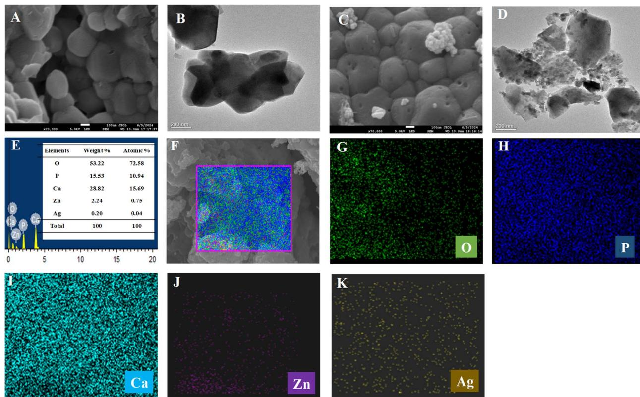
Fig. 3 (A and B) Morphology of the synthesized HAP via SEM and TEM. (C and D) Surface morphology of the Ag-ZnO@HAP nanocomposite via SEM and TEM. (E and the inset table) Elemental composition and their percentages present in Ag-ZnO@HAP. (F-K) Elemental mapping of the synthesized nanocomposite, showing a uniform distribution of the doped elements.
