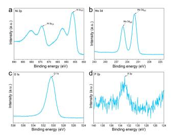
Fig. 5 XPS spectrum of (a) Ni 2p, (b) Mo 3d, (c) O 1s and (d) P 2p moieties of PMA-Ni(OH)<sub>2</sub> crumpled nanosheets.
