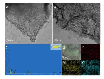
Fig. 1 (a and b) TEM images at different magnifications, (c) EDX spectrum and (d) Elemental mapping through EDX of PMA-Ni(OH)<sub>2</sub> flexible nanosheets.
