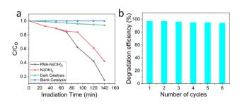
Fig. 7 (a) Photodegradation of MB dyes under different conditions (b) stability test of PMA-Ni(OH)<sub>2</sub> through recycling experiments.
