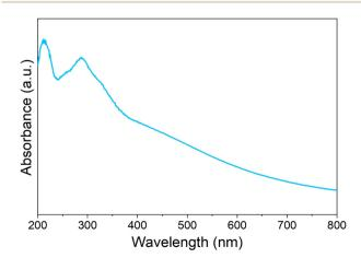
Fig. 6 UV-visible spectrum of PMA-Ni(OH)<sub>2</sub> flexible nanosheets.
