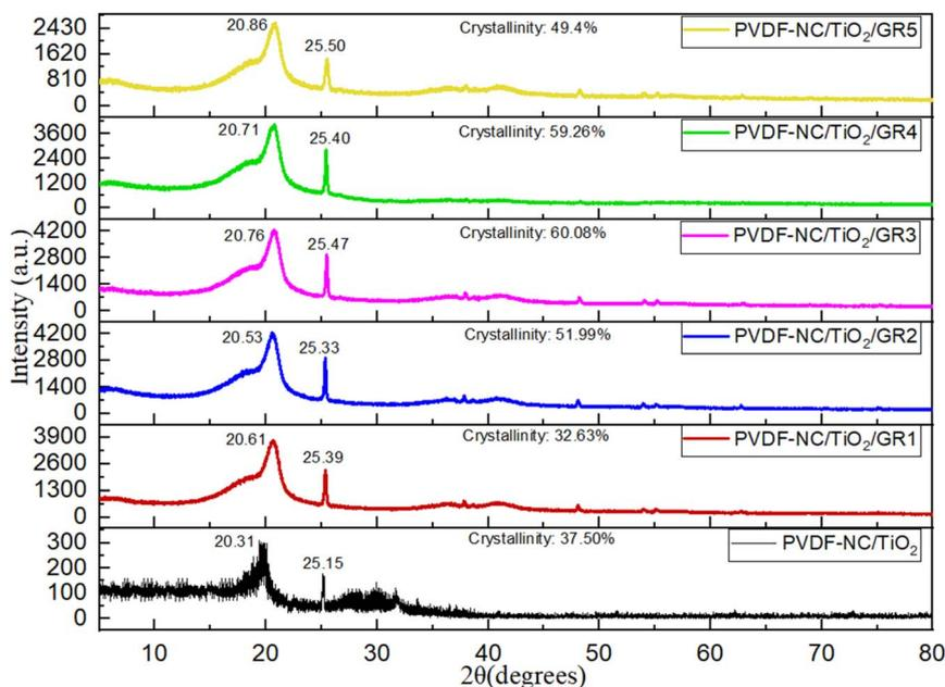
Fig. 2 The XRD patterns of the reference PVDF-NC/TiO<sub>2</sub> membrane and the graphene-incorporated PVDF-NC/TiO<sub>2</sub> membranes with varying graphene loading percentages.
