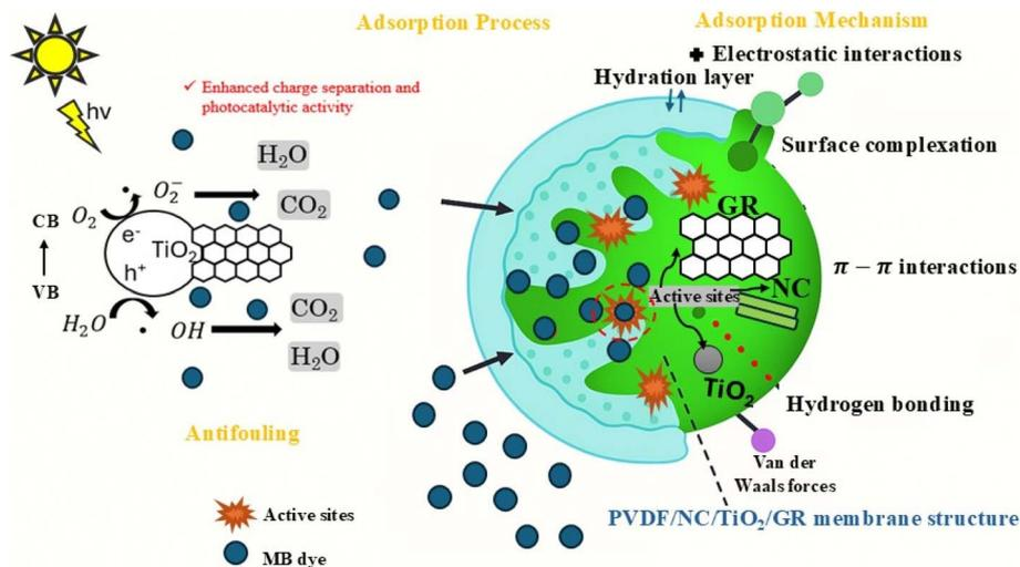
Fig. 6 Schematic illustration of antifouling, adsorption and photocatalytic mechanisms of the PVDF-NC/TiO<sub>2</sub>/GR nanocomposite membrane for MB dye removal.
