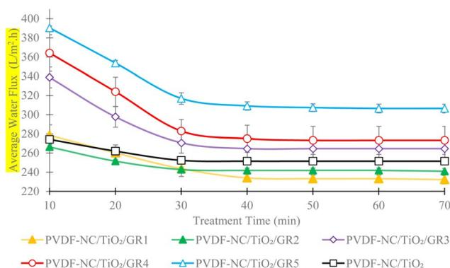
Fig. 3 Comparative water flux analysis of PVDF/NC/TiO<sub>2</sub>/GR nanocomposite membranes with varying graphene loading percentages relative to the control PVDF/NC/TiO<sub>2</sub> membrane.
