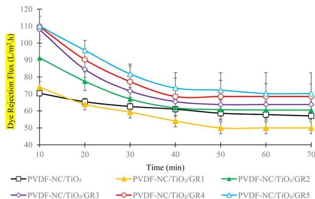
Fig. 4 Comparative dye rejection analysis of PVDF/NC/TiO<sub>2</sub>/GR nanocomposite membranes with varying graphene loading percentages relative to the control PVDF/NC/TiO<sub>2</sub> membrane.
