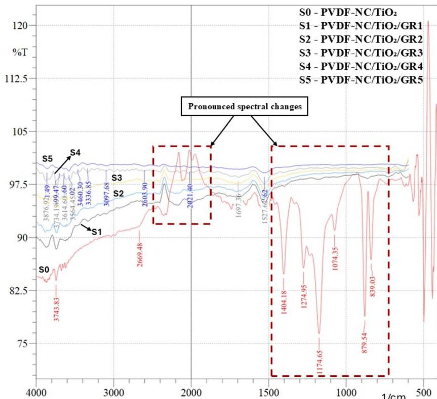
Fig. 1 FTIR spectra of the control nanocomposite membrane (PVDF-NC/TiO<sub>2</sub>) and GR-incorporated nanocomposite membranes (PVDF-NC/TiO<sub>2</sub>/GR) with varied GR loadings.
