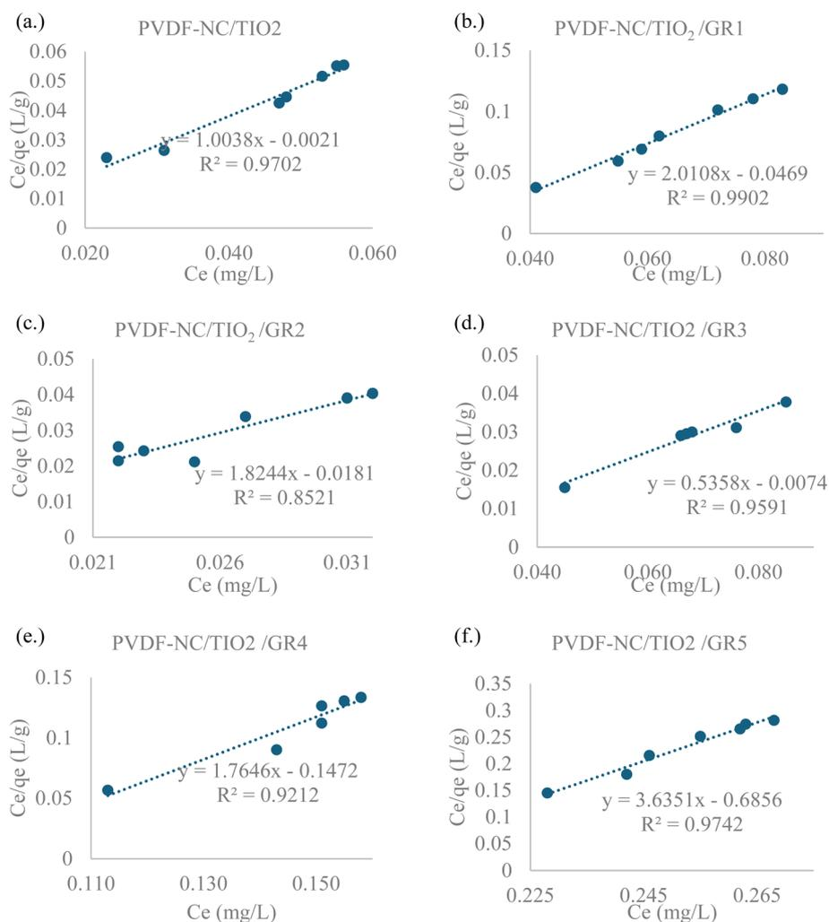
Fig. 7 Linearized Langmuir isotherm plots for MB dye adsorption onto (a) PVDF-NC/TiO<sub>2</sub>, (b) PVDF-NC/TiO<sub>2</sub>/GR1, (c) PVDF-NC/TiO<sub>2</sub>/GR2, (d) PVDF-NC/TiO<sub>2</sub>/GR3, (e) PVDF-NC/TiO<sub>2</sub>/GR4, (f) PVDF-NC/TiO<sub>2</sub>/GR5 nanocomposite membranes at 25 °C.
