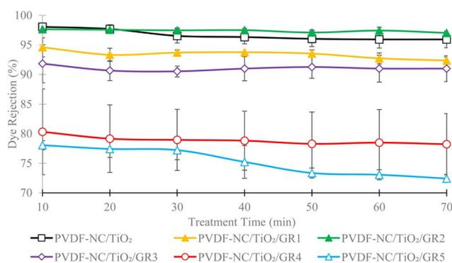
Fig. 5 Analysis of MB dye removal percentages of PVDF/NC/TiO<sub>2</sub>/GR nanocomposite membranes with varying graphene loading percentages relative to the control PVDF/NC/TiO<sub>2</sub> membrane.
