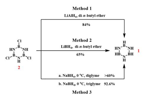
Scheme 2 Routes for the reduction of *B*-trichloroborazine to borazine.<sup>76,77</sup>
