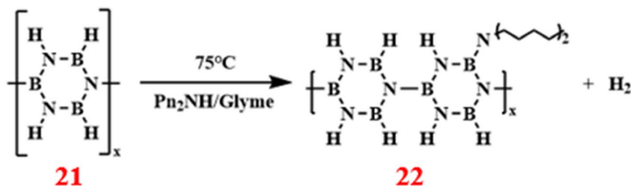
Scheme 16 Synthesis route of dipentylamine-modified polyborazine. 89
