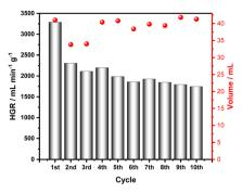
Fig. 7 Evaluation of different catalytic cycles in hydrogen evolution from  $NH_3BH_3$  mediated by  $PtNPs/LiNbWO_6$ . Conditions: 20 mg of support, 3 mmol% of PtNPs, 0.58 mmol of  $NH_3BH_3$ , and temperature: 27 °C.
