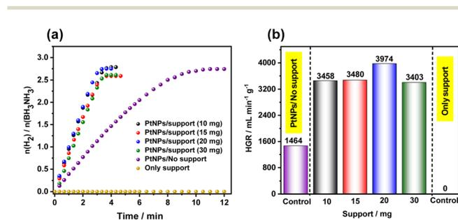
Fig. 4 (a) Evaluation of the influence of LiNbWO<sub>6</sub> support on hydrogen evolution from NH<sub>3</sub>BH<sub>3</sub> (b) HGR for different amounts of support. Conditions: 0.58 mmol of ammonium borane, 3 mmol% of Pt NPs, temperature: 27 °C.
