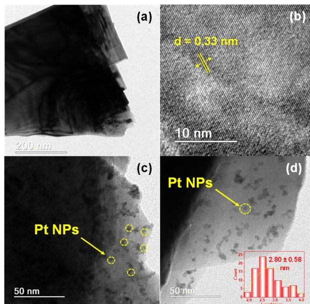
Fig. 2 Transmission electron microscopy (TEM) images of  $\text{LiNbWO}_6$  (a) and (b);  $\text{PtNPs}/\text{LiNbWO}_6$  (c) and (d) with insert showing the PtNPs size distribution.
