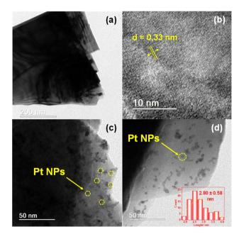
Fig. 2 Transmission electron microscopy (TEM) images of LiNbWO<sub>6</sub> (a) and (b); PtNPs/LiNbWO<sub>6</sub> (c) and (d) with insert showing the PtNPs size distribution.
