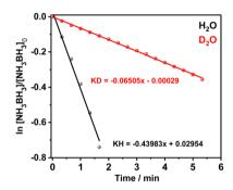
Fig. 5 Evaluation of the Kinetic Isotope Effect (KIE) in  $H_2O$  and  $D_2O$  during the hydrogen evolution reaction from NH<sub>3</sub>BH<sub>3</sub>. Conditions: support (20 mg); PtNPs/LiNbWO<sub>6</sub> catalyst (3.00 mmol%); NH<sub>3</sub>BH<sub>3</sub> (0.500 mol L<sup>-1</sup>).
