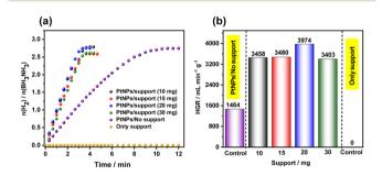
Fig. 4 (a) Evaluation of the influence of LiNbWO $_6$  support on hydrogen evolution from NH $_3$ BH $_3$  (b) HGR for different amounts of support. Conditions: 0.58 mmol of ammonium borane, 3 mmol% of Pt NPs, temperature: 27 °C.
