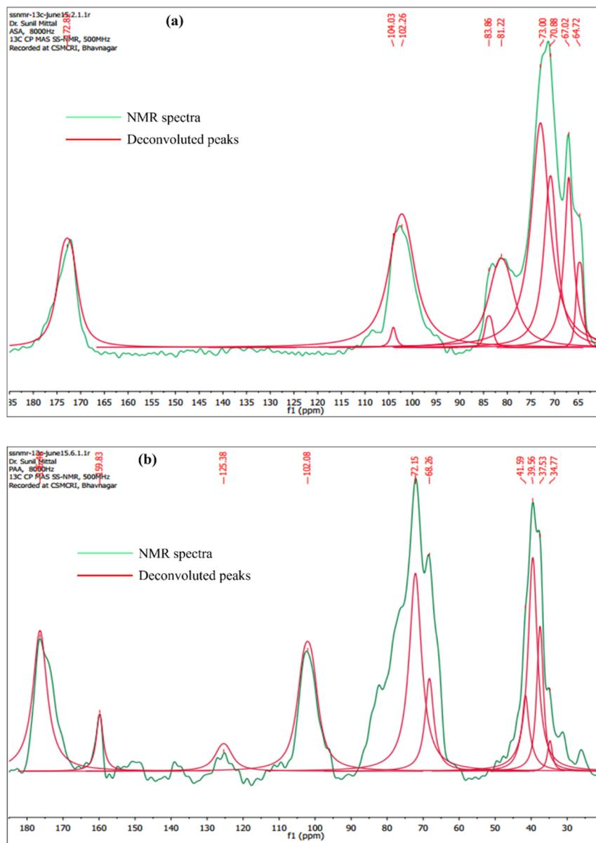
Fig. 2 Global Spectral Deconvolution of CP-MAS <sup>13</sup>C NMR spectrum of (a) AA; and (b) PAA.
