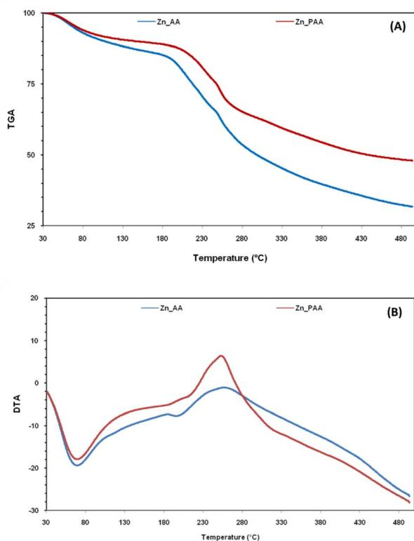
Fig. 12 (a) Thermo-gravimetric analysis; and differential thermal analysis (DTA) of Zn adsorbed samples of AA and PAA.
