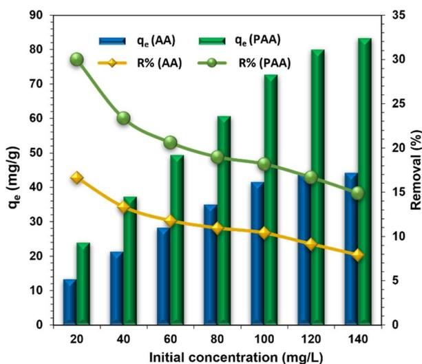
Fig. 6 Effect of change in initial Zn(II) concentrations on the adsorptive removal efficiencies of AA and PAA.  $\{[\text{Adsorbent}] = 0.25 \text{ g L}^{-1}, \text{pH} = 25 \pm 1^\circ \text{C}, \text{time} = 2 \text{ h}, \text{shaking speed} = 200 \text{ rpm}, \text{equilibrium time} = 22 \text{ h}\}$ .
