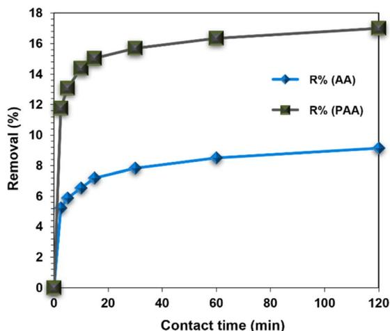
Fig. 8 Effect of contact time on % removal of Zn(II) by AA and PAA ( $[Zn(II)] = 100 \text{ mg L}^{-1}$ ,  $\text{pH} = 5$ ,  $[\text{Adsorbent}] = 0.25 \text{ g L}^{-1}$ ,  $\text{temp.} = 25 \pm 1^\circ \text{C}$ , shaking speed = 200 rpm).
