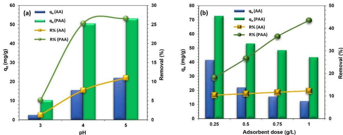
Fig. 5 Effect of (a) pH; and (b) adsorbent dose on the removal of Zn(II) by AA and PAA.  $\{[Zn^{2+}] = 100 \text{ mg L}^{-1}; [\text{adsorbent}] = 0.5 \text{ g L}^{-1}; \text{temp.} = 25 \pm 1^\circ \text{C}, \text{time} = 2 \text{ h}, \text{shaking speed} = 200 \text{ rpm}, \text{equilibrium time} = 22 \text{ h}\}$ .
