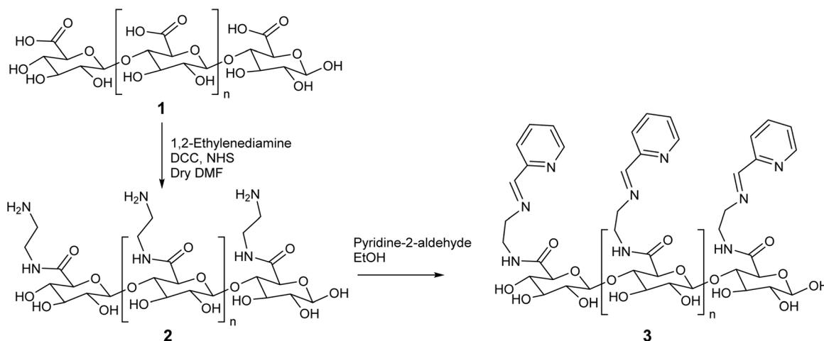
Scheme 1 Schematic representation for synthesis of PAA.
