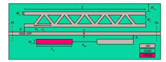
Fig. 1 2D layout of the designed sensor
