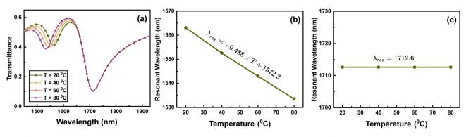
Fig. 10 (a) Transmittance profile of the proposed sensor under varying temperatures of PDMS. (b) Graph of resonant wavelength *versus* temperature for mode 1. (c) Graph of resonant wavelength *versus* temperature for mode 2.
