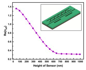
Fig. 3 Variation of the real part of the effective refractive index  $(Re(n_{eff}))$  with the height of the 3D simulated structure, indicating the quasi-2D behavior.
