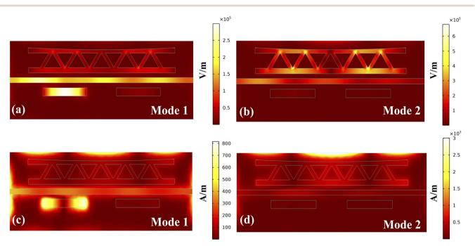
Fig. 8 (a) E-field at mode 1 after deformation. (b) E-field at mode 2 after deformation. (c) H-field at mode 1 after deformation. (d) H-field at mode 2 after deformation. 2 after deformation.
