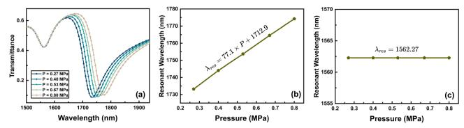
Fig. 9 (a) Transmittance profile of the proposed sensor under varying applied pressure. (b) Graph of the resonant wavelength versus pressure for mode 2. (c) Graph of resonant wavelength versus pressure for mode 1.
