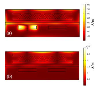
Fig. 6 H-field at (a)  $\lambda_{res} = 1562.9$  nm (mode 1), (b)  $\lambda_{res} = 1712.2$  nm (mode 2).
