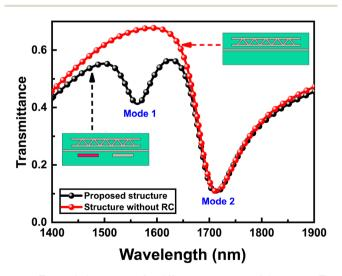
Fig. 4 Transmission spectra for different structures of the sensor. The black graph represents the results for the proposed sensor and the red graph represents the spectrum for the structure without RCs.
