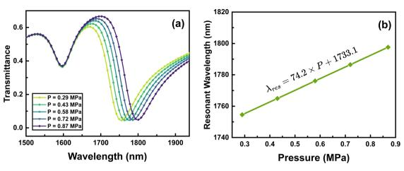
Fig. 13 (a) Transmittance profile of the proposed sensor with silver incorporated, under varying applied pressure. (b) Graph of resonant wavelength *versus* pressure for mode 2.
