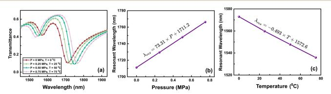
Fig. 11 (a) Transmission profile of the proposed sensor while performing dual-sensing under different pressures and temperatures. (b) Resonant wavelength *versus* pressure for mode 2. (c) Resonant wavelength *versus* temperature for mode 1.
