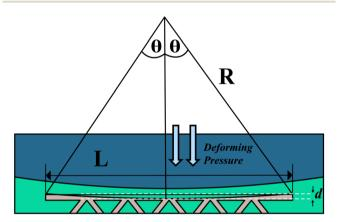
Fig. 7 Formation of an arc in the resonator with a deformation (d) due to the exerted pressure.
