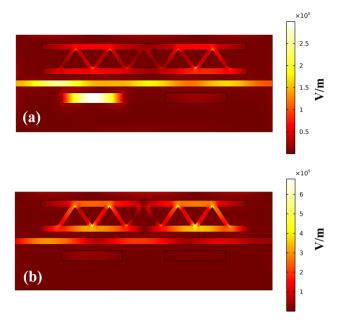
Fig. 5 E-field at (a)  $\lambda_{res} = 1562.9$  nm (mode 1), (b)  $\lambda_{res} = 1712.2$  nm (mode 2).
