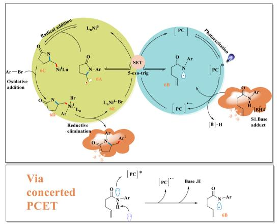
Scheme 6 Proposed catalytic cycle with PCET mechanism.
