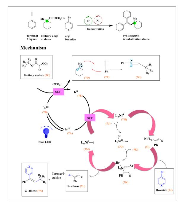
Scheme 7 A suggested method for using photoredox and nickel catalysts to syn-selectively alkylate terminal alkynes.
