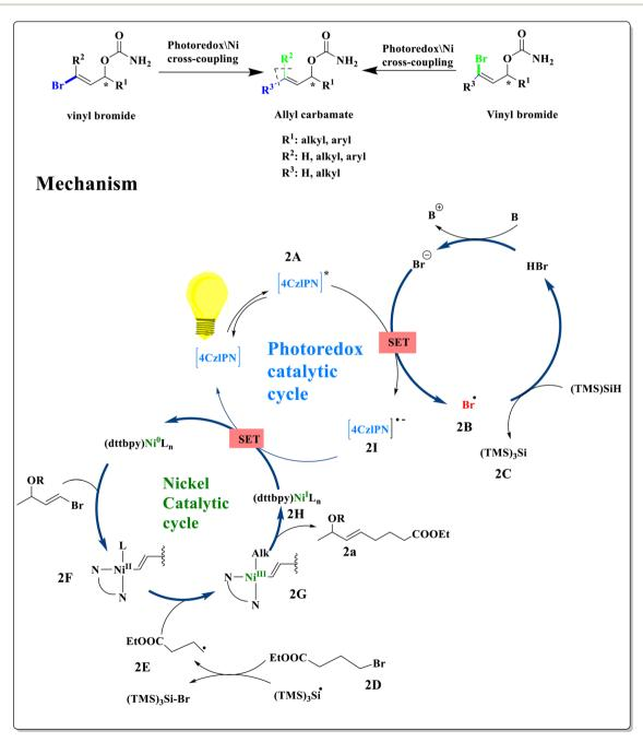
Scheme 2 Proposed mechanism for photocatalytic alkenylation of vinyl bromides. <sup>a</sup> L= ligand.
