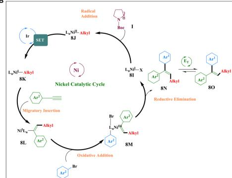
Scheme 8 (a) Proposed mechanism for the hydroalkylation of alkynes by photoredox and nickel dual catalysis. (b) A proposed mechanism for the arylalkylation of alkynes by photo/nickel dual catalysis.
