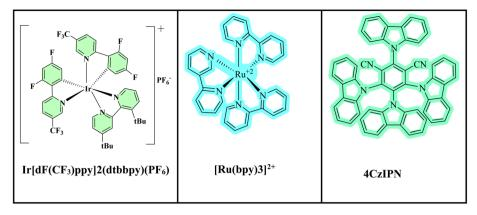
Fig. 1 Some photocatalysts used in dual catalysis.
