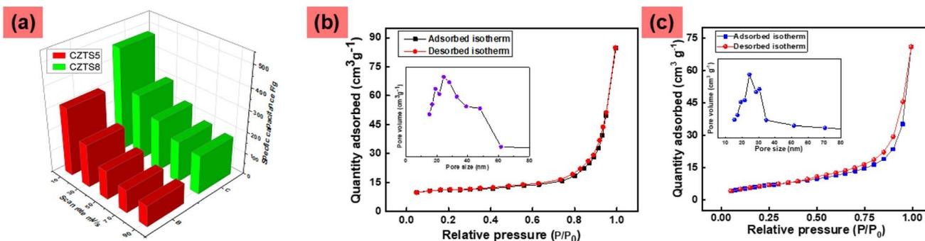
Fig. 8 (a) Presents a specific capacitance *versus* scan rate plot for CZTS5 and CZTS8 electrodes, the nitrogen adsorption–desorption isotherms, and (inset) the pore size distribution of CZTS5 (b), and CZTS8 (c).
