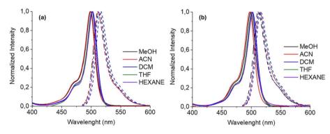
Fig. 24 Absorption (solid line) and emission (dotted line) spectra of (a) conjugate 92 and (b) conjugate 95 in different solvents. Reproduced with permission from ref. 100. Copyright 2019, Springer Nature.
