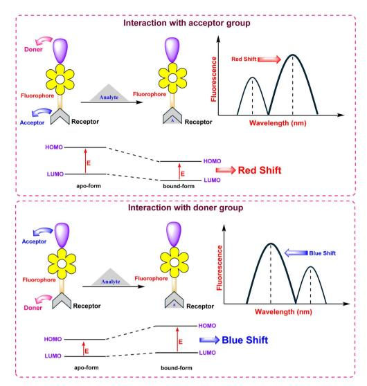
Fig. 13 Mechanism of intramolecular charge transfer (ICT).
