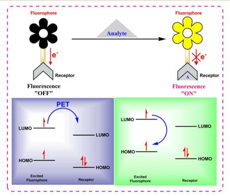
Fig. 12 Mechanism of photoinduced electron transfer (PET).
