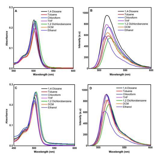
Fig. 25 (a) Absorption spectra of conjugate **96** in different solvents; (b) emission spectra of conjugate **96** in different solvents; (c) absorption spectra of conjugate **98** in different solvents. Reproduced with permission from ref. 101. Copyright 2020, Royal Society of Chemistry.
