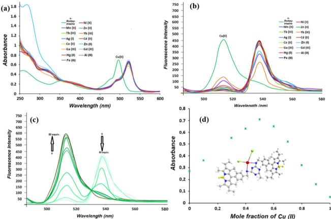
Fig. 17 (a) Absorbance spectra of conjugate 30 with various metal ions; (b) fluorescence spectra of conjugate 30 with various metal ions; (c) Cu(III) titration of conjugate 30 at different concentrations in DMF/H<sub>2</sub>O; (d) Job's Plot of conjugate 30/Cu(III) reproduced with permission from ref. 86. Copyright 2014, Elsevier.
