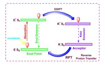
**Fig. 15** Mechanism of excited-state intramolecular proton transfer (ESIPT).
