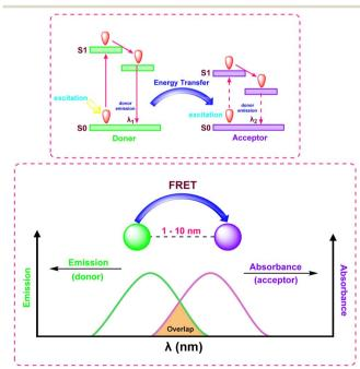
Fig. 14 Mechanism of fluorescence resonance energy transfer (FRET).
