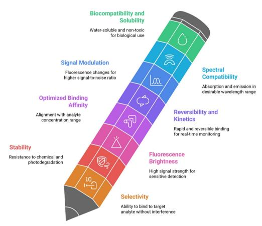
Fig. 11 Design criteria for fluorescent sensors.
