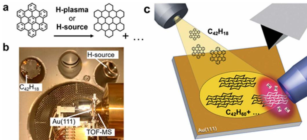
Fig. 52 (a) Hydrogenation of HBC nanographene in the direction of an archetype ((b) and (c)) Au(111) sample at the EI-TOF-MS measurement location within the chamber. Reproduced from ref. 221 with permission from American Chemical Society, Copyright © 2023.
