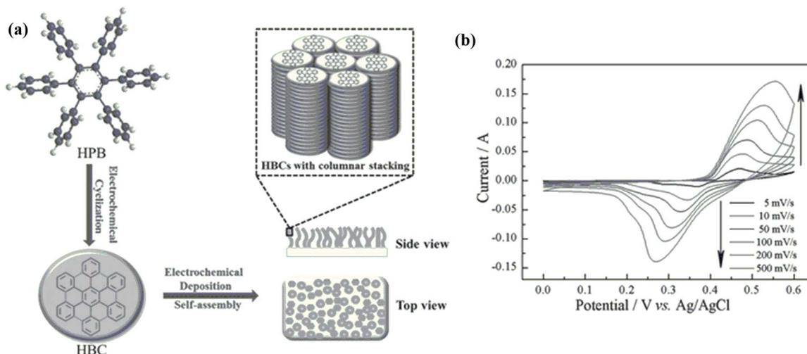
Fig. 44 (a) Diagram showing the assembling of HBC on an electrode and its *in situ* electrochemical production. (b) Representative cyclic voltammograms of the HBC assembly on ITO, obtained in a 6 M KOH solution at different scan speeds between 5 and 500  $\text{mV s}^{-1}$ . Reproduced from ref. 208 with permission from John Wiley & Sons, Copyright © 2015, Wiley-VCH Verlag GmbH & Co. KGaA, Weinheim.
