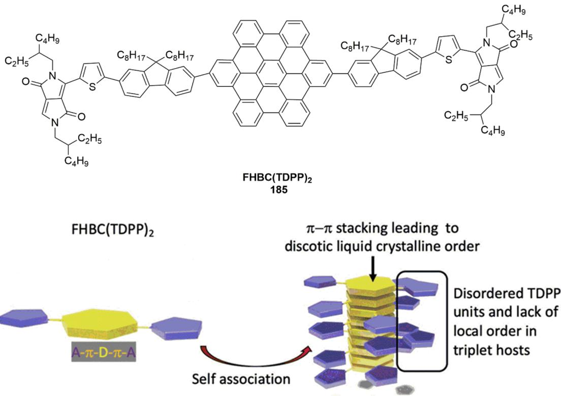
Fig. 58 The chemical structure of FHBC(TDPP)<sub>2</sub> (**185**) is characterized by an acceptor- $\pi$ -donor- $\pi$ -acceptor (A- $\pi$ -D- $\pi$ -A) configuration, where the central HBC moiety functions as the electron-donating core (D). Reproduced from ref. 226 with permission from John Wiley & Sons, Copyright © 2019, Wiley-VCH Verlag GmbH & Co. KGaA, Weinheim.
