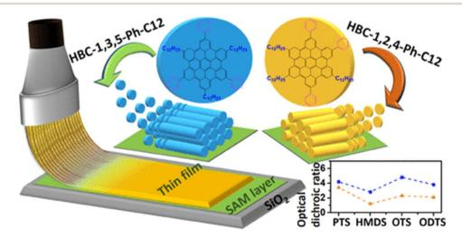
Fig. 41 Graphical representation of brush-coated molecularly aligned HBCs films and application in thin-film transistors. Reproduced from ref. 205 with permission from American Chemical Society, Copyright © 2019.
