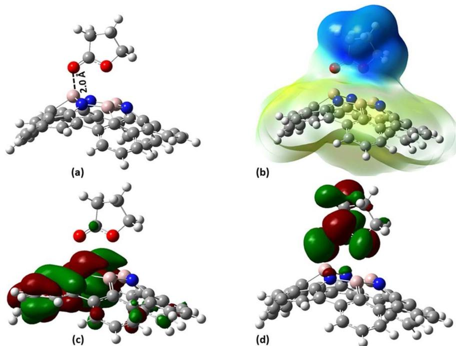
Fig. 50 AlN-HBC:GBL complex's (a) optimized structure, (b) MEP, (c) HOMO, and (d) LUMO profiles. Distances are measured in Å. Reproduced from ref. 219 with permission from Elsevier, Copyright © 2021.
