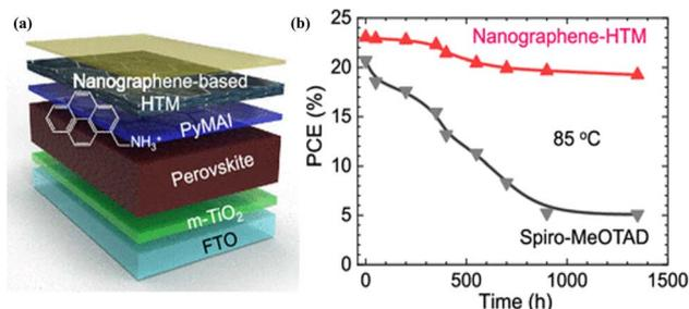
Fig. 64 (a) The FTO/*m*-TiO<sub>2</sub>/perovskite/HTM/Au device structure is shown schematically, with PyMAI acting as an interface modifier between the perovskite and HBC-DPA(Me)OMe (b) PCE using the ISOS-D-2I protocol as a function of aging time at 85 °C. Reproduced from ref. 232 with permission from American Chemical Society, Copyright © 2023.
