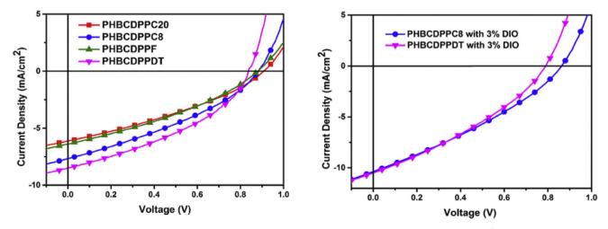
$Fig.~39~~(Left)~Current~density-voltage~characteristics~of~polymer/PC_{71}BM-based~PSCs~with~AM~1.5~G,~100~mW~cm^{-2}~illumination~(right)~features$ of the current density and voltage of PSC devices of PHBCDPPC8 and PHBCDPPDT following processing with DIO additive under 100 mW cm $^{-2}$ of AM 1.5 G illumination. Reproduced from ref. 203 with permission from Elsevier, Copyright © 2016.
