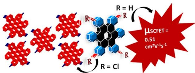
Fig. 42 Graphical representation of polysubstituted hexa-*cata*-HBC and its applications in transistors. Reproduced from ref. 206 with permission from American Chemical Society, Copyright © 2019.
