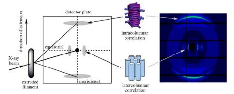
Fig. 23 Diagrammatic illustration of the experimental assembly (left) and 2D WAXS pattern of HBC scaffold 28 represent intra- and intercolumnar organization (right). Reproduced from ref. 184 with permission from American Chemical Society, Copyright © 2005.
