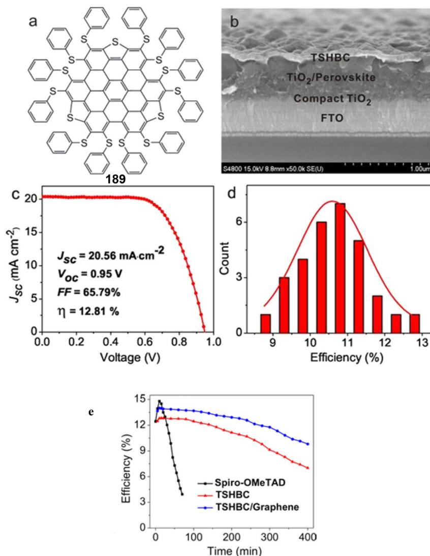
Fig. 62 (a) The molecular representation of TSHBC. (b) SEM image of the device of FTO/TiO<sub>2</sub>/perovskite/TSHBC film. The best *I*-*V* characteristics (c) comparison of the performance distributions of 30 individual devices (d) of the cells. (e) The efficiency variation of the devices stored under illumination at AM 1.5 G with the humidity of 45%. Reproduced from ref. 230 with permission from American Chemical Society, Copyright © 2015.
