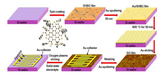
Fig. 45 Diagrammatic representation of SG films for planar MSCs on a  $Si/SiO_2$  wafer produced from SHBC. Reproduced from ref. 209 with permission from American Chemical Society, Copyright © 2017.
