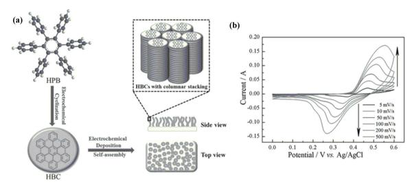
Fig. 44 (a) Diagram showing the assembling of HBC on an electrode and it's *in situ* electrochemical production. (b) Representative cyclic voltammograms of the HBC assembly on ITO, obtained in a 6 M KOH solution at different scan speeds between 5 and 500 mV s<sup>-1</sup>. Reproduced from ref. 208 with permission from John Wiley & Sons, Copyright © 2015, Wiley-VCH Verlag GmbH & Co. KGaA, Weinheim.
