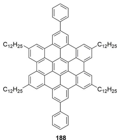
Fig. 61 Molecular structure of HBC-1,3,5-Ph-C<sub>12</sub>.<sup>229</sup>
