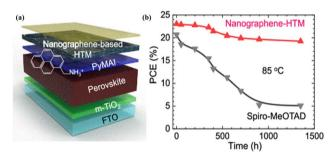
Fig. 64 (a) The FTO/m-TiO<sub>2</sub>/perovskite/HTM/Au device structure is shown schematically, with PyMAI acting as an interface modifier between the perovskite and HBC-DPA(Me)OMe (b) PCE using the ISOS-D-2I protocol as a function of aging time at 85 °C. Reproduced from ref. 232 with permission from American Chemical Society, Copyright © 2023.
