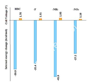
Fig. 47 Li-ion battery cell voltage and the plot of eternal energy change for Li and Li<sup>+</sup> adsorption on various HBC-based nanosheets. Reproduced from ref. 212 with permission from Elsevier, Copyright © 2020.
