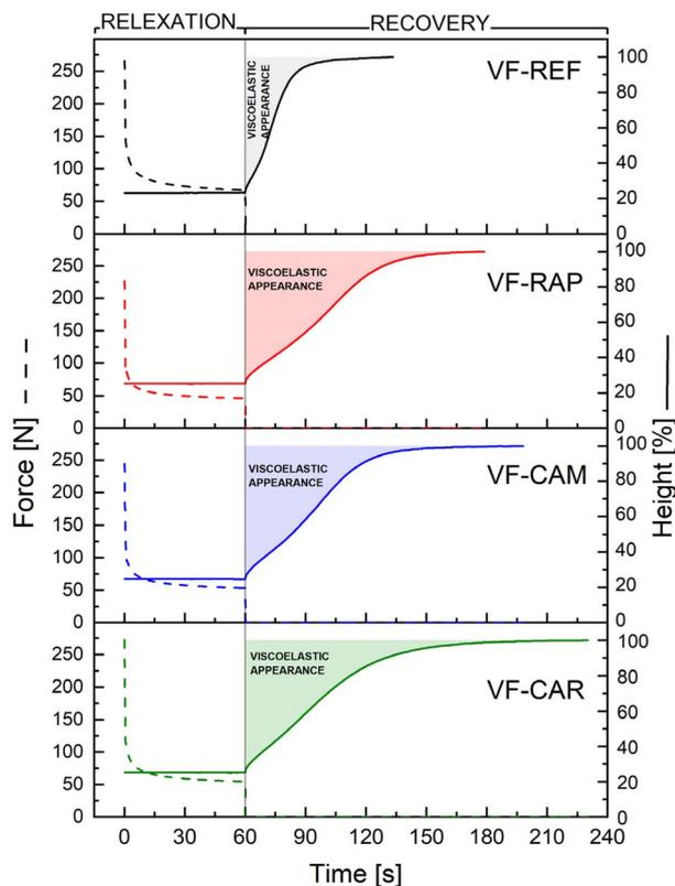
Fig. 6 Viscoelastic properties of the foams measured with RESIMAT®.
