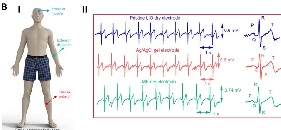
Fig. 7 (A) Schematic image related to the fabrication of LIG/MXene-Ti<sub>3</sub>C<sub>2</sub>T<sub>x</sub>@EDOT sensor. (B) Schematic image related to measurement of temperature from strain-insensitive of body parts (I). Utilizing different electrodes (including Ag/AgCl gel, LIG, and LIG/MXene-Ti<sub>3</sub>C<sub>2</sub>T<sub>x</sub>@EDOT electrodes) for checking ECG (II). Reprinted with permission from ref. 114. Copyright 2022, Nature.
