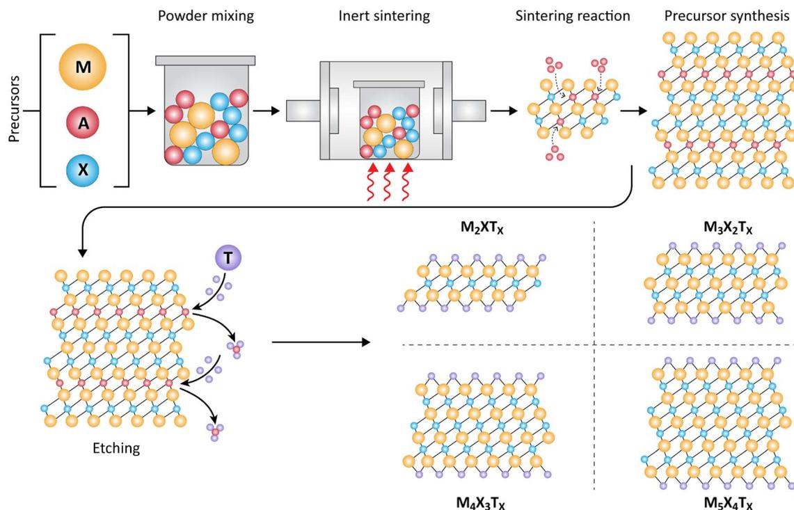
Fig. 5 Synthesis and chemical structure of MXenes.
