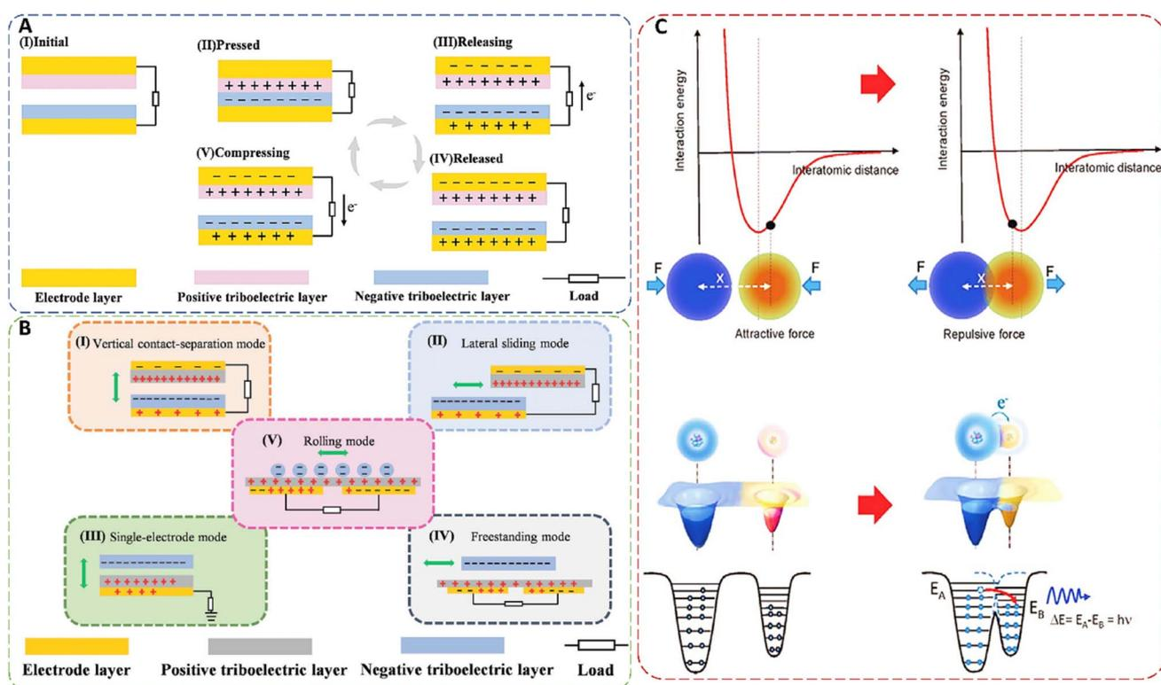
Fig. 1 (A) The mechanism of TENG's working, including (I) initial, (II) pressed, (III) releasing, (IV) released, and (V) compressing. (B) Five basic modes of TENGs: (I) vertical contact-separation mode. (II) Lateral sliding mode. (III) Single-electrode mode. (IV) Freestanding mode. (V) Rolling mode. (C) Explaining the contact electrification (CE) model and how charge transfers between two atoms. Reprinted with permission from ref. 37. Copyright 2024, Wiley-VCH GmbH.
