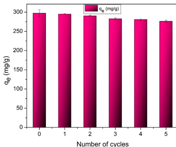
Fig. 12 Regeneration-reuse of FCOB for CV adsorption up to five cycles.
