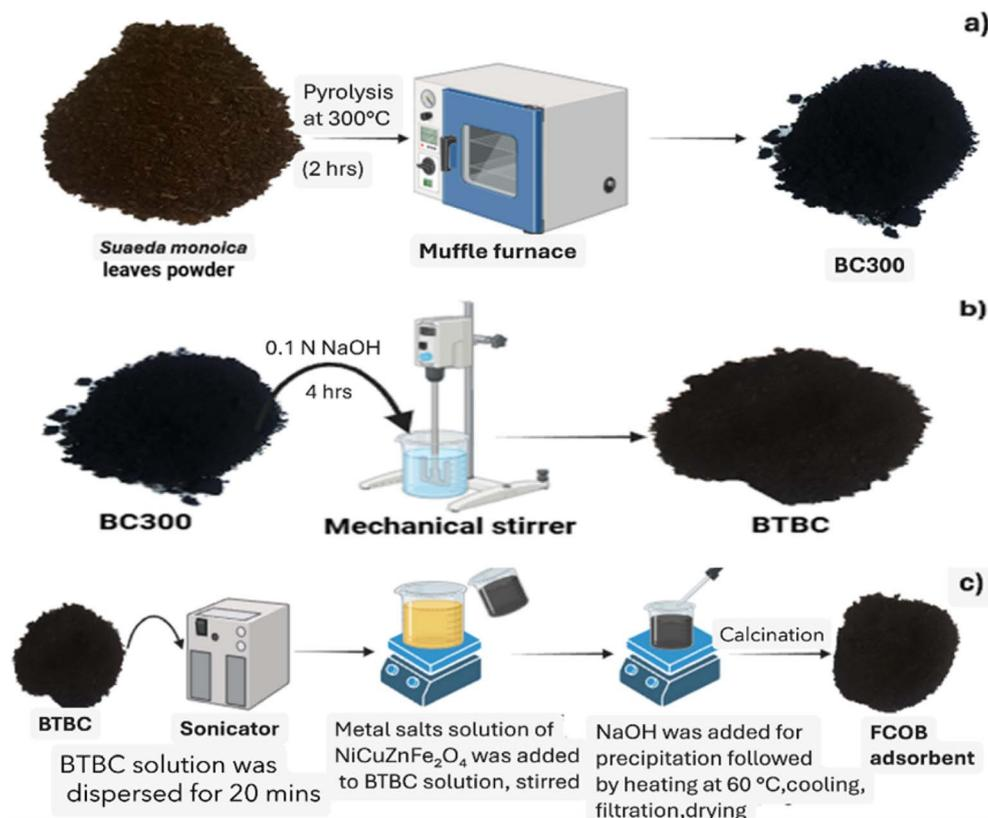
Fig. 1 Synthesis of FCOB adsorbent.
