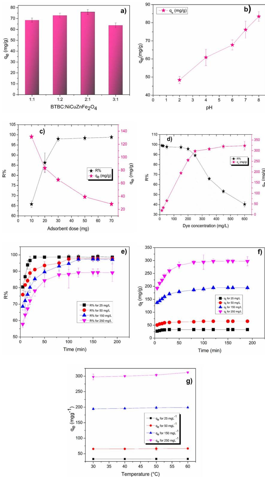
Fig. 9 Effect of different parameters on the adsorption of CV by FCOB: (a) BTBC : NiCuZnFe<sub>2</sub>O<sub>4</sub> content, (b) pH, (c) adsorbent dose, (d) initial dye concentration, (e–f) contact time, and (g) temperature.
