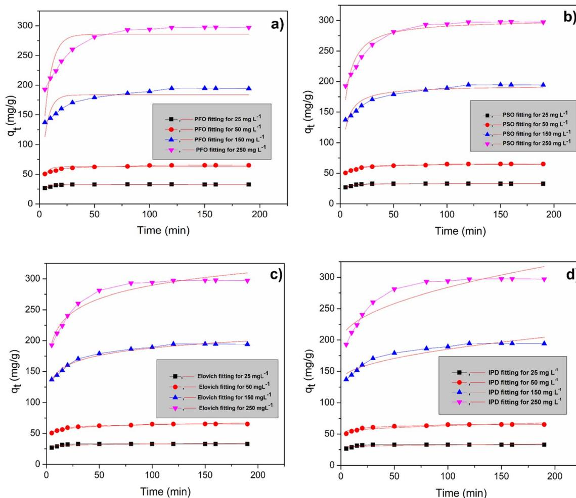
Fig. 10 Non-linear kinetic fitting of CV adsorption onto FCOB: (a) PFO, (b) PSO, (c) Elovich, and (d) IPD at 25–250 mg L<sup>-1</sup> initial concentrations.
