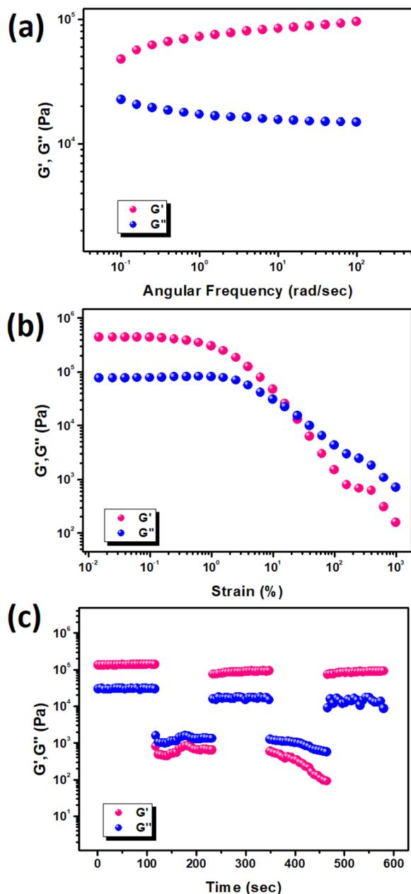
Fig. 2 (a) Angular frequency measurements vs.  $G'$  and  $G''$  of NiC-GT metalhydrogel; (b) strain-sweep measurements of NiC-GT metalhydrogel performed at a constant frequency of 6.283 rad s<sup>-1</sup>; (c) thixotropic measurement performed on the NiC-GT metalhydrogel, examining its thixotropic behavior.
