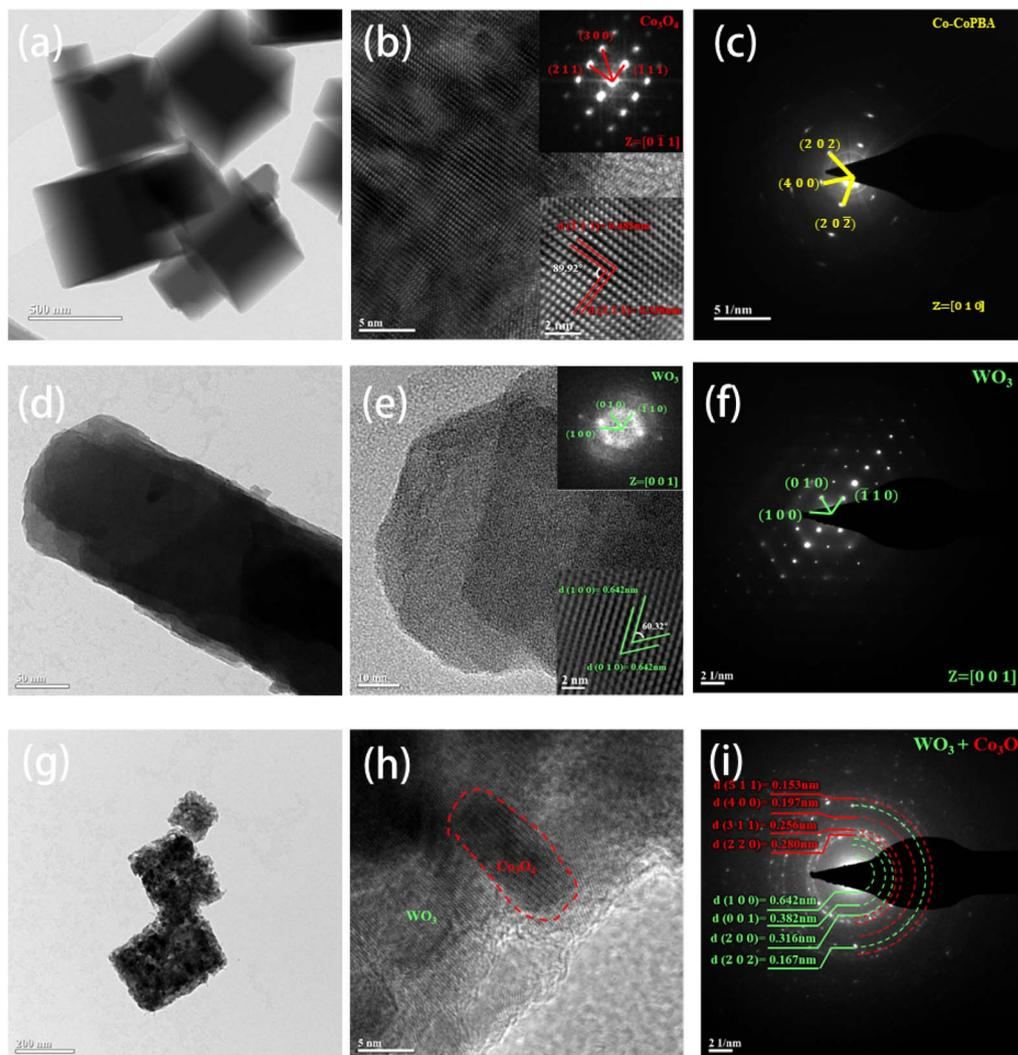
Fig. 2 (a) TEM images of Co-CoPBA; (b) high-resolution images; (c) electron diffraction images; (d) TEM images of  $\text{WO}_3$ ; (e) high-resolution images; (f) electron diffraction images; (g) TEM images of  $\text{WO}_3$ @Co-CoPBA-500 °C; (h) high-resolution images; (i) electron diffraction pattern.
