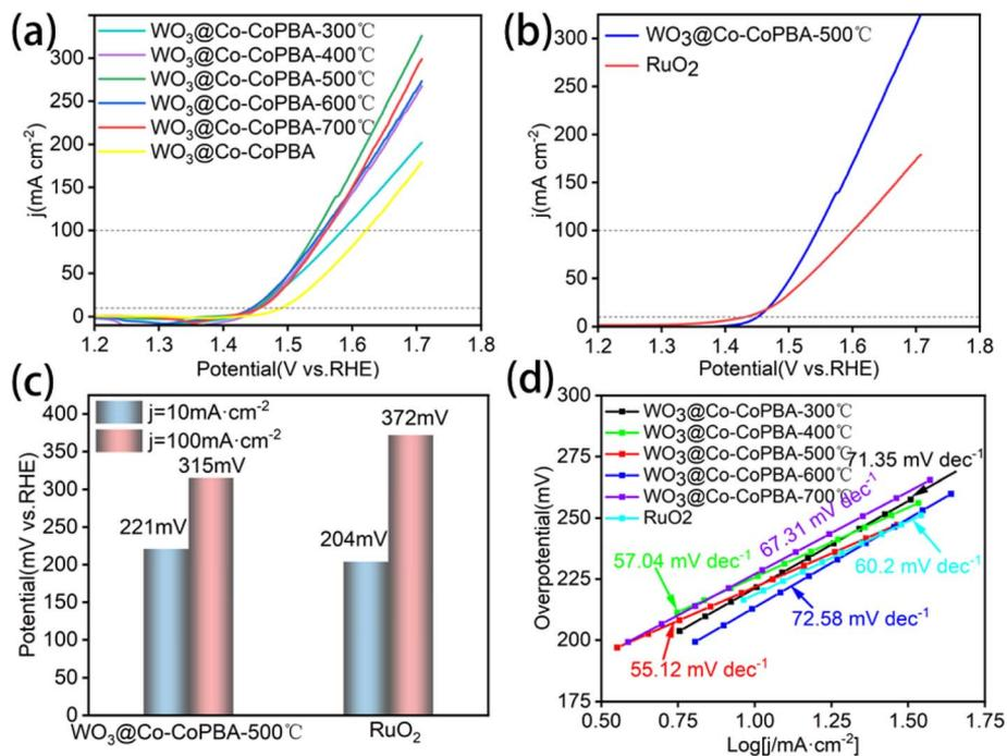
Fig. 4 (a) LSV curves for different annealing temperatures; (b) LSV curves for WO<sub>3</sub>@Co-CoPBA-500 °C versus RuO<sub>2</sub>; (c) Overpotentials at different current densities; (d) Tafel curves for test samples.
