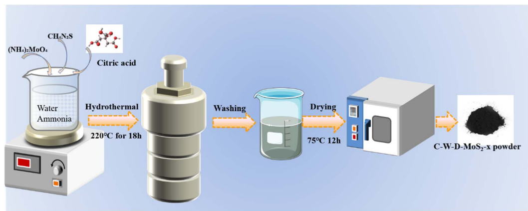
Fig. 1 The process diagram of C-W-D-MoS 2 -x.
