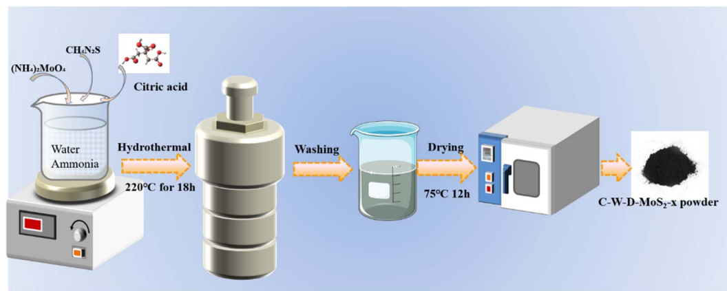
Fig. 1 The process diagram of C-W-D-MoS 2-x .
