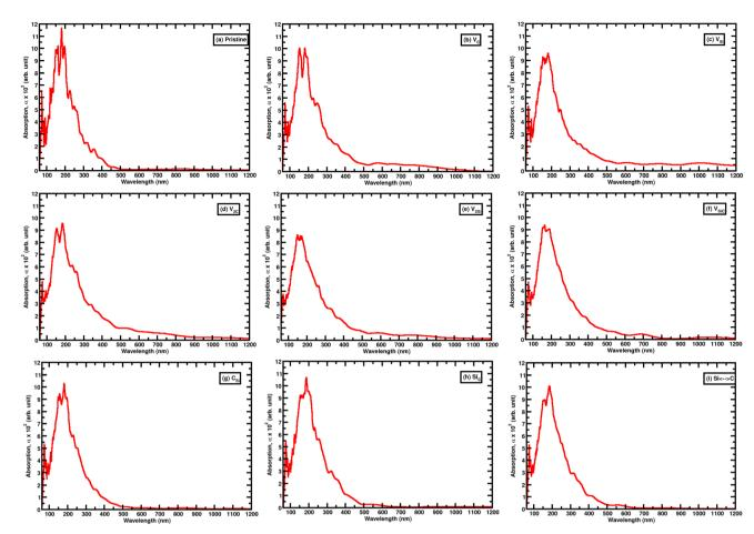
Fig. 13 (a) The absorption coefficient of pristine monolayer SiC; the absorption coefficient of single vacancy defect in a monolayer of SiC: (b)  $V_C$ , (c)  $V_{Si}$ ; the absorption coefficient of double vacancy defect in a monolayer of SiC: (d)  $V_{2C}$ , (e)  $V_{2Si}$ , (f)  $V_{SiC}$ ; the absorption coefficient of antisite defect in a monolayer of SiC: (g)  $C_{Si}$ , (h)  $Si_C$ , (i)  $Si \leftrightarrow C$ .
