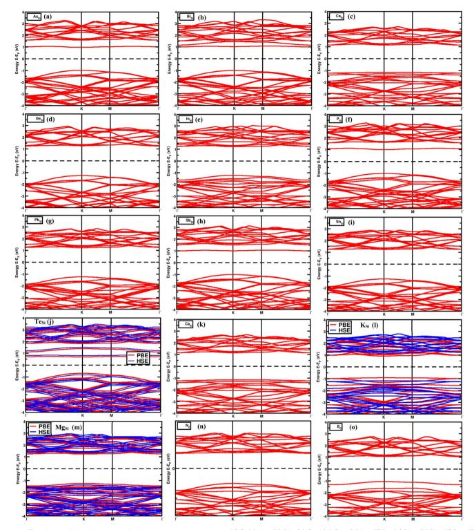
Fig. 6 The electrical band diagrams of point doping in a monolayer of SiC: (a)  $As_{Si}$ , (b)  $Bi_{Si}$ , (c)  $Ga_{Si}$ , (d)  $Ge_{Si}$ , (e)  $In_{Si}$ , (g)  $Pb_{Si}$ , (h)  $Sb_{Si}$ , (i)  $Sn_{Si}$ , (j)  $Te_{Si}$ , (k)  $Ca_{Si}$ , (l)  $K_{Si}$ , (m)  $Mg_{Si}$ , (n)  $N_{C}$ , (o)  $B_{C}$ .
