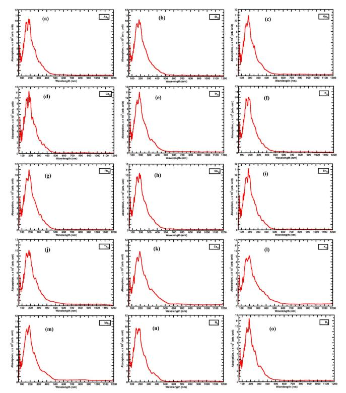
Fig. 14 The absorption coefficient of point doping in a monolayer of SiC: (a) As<sub>Si</sub>, (b) Bi<sub>Si</sub>, (c) Ga<sub>Si</sub>, (d) Ge<sub>Si</sub>, (e) In<sub>Si</sub>, (f) P<sub>Si</sub>, (g) Pb<sub>Si</sub>, (h) Sb<sub>Si</sub>, (i) Sn<sub>Si</sub>, (j)  $Te_{Si}$ , (k)  $Ca_{Si}$ , (l)  $K_{Si}$ , (m)  $Mg_{Si}$ , (n)  $N_{C}$ , (o)  $B_{C}$ .
