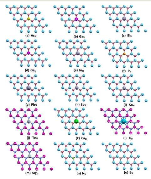
Fig. 2 The structural configuration of point doping in a monolayer of SiC: (a) As<sub>Si</sub>, (b) Bi<sub>Si</sub>, (c) Ga<sub>Si</sub>, (d) Ge<sub>Si</sub>, (e) In<sub>Si</sub>, (f) P<sub>Si</sub>, (g) Pb<sub>Si</sub>, (h) Sb<sub>Si</sub>, (i) Sn<sub>Si</sub>, (j)  $Te_{Si}$ , (k)  $Ca_{Si}$ , (l)  $K_{Si}$ , (m)  $Mg_{Si}$ , (n)  $N_C$ , (o)  $B_C$ .
