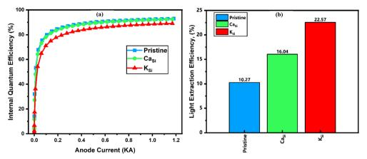
Fig. 19 (a) Variation of internal quantum efficiency as a function of anode current for the proposed LED utilizing pristine SiC, K<sub>Si</sub>, and Ca<sub>Si</sub> as an active layer; (b) the light extraction efficiency of proposed LEDs.
