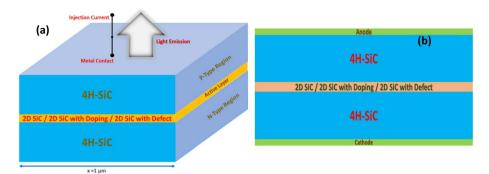
Fig. 3 A schematic of SiC-based light-emitting diode: (a) 3D view; (b) cross-section of the front view.
