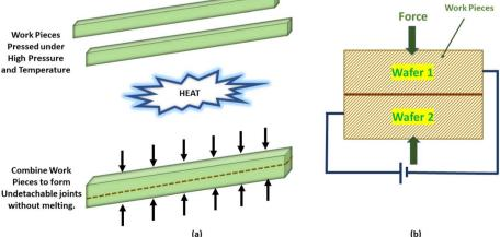
Fig. 4 Process diagram for diffusion welding (a) two wafers bonded together at high heat and pressure; (b) wafers 1 and 2 bonded directly together at high pressure.<sup>105</sup>
