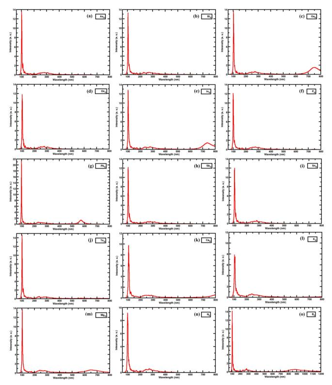
Fig. 16 The electron energy loss spectrum of point doping in a monolayer of SiC: (a)  $As_{Si}$ , (b)  $Bi_{Si}$ , (c)  $Ga_{Si}$ , (d)  $Ge_{Si}$ , (e)  $In_{Si}$ , (f)  $Ps_{Si}$ , (h)  $Sb_{Si}$ , (i)  $Sb_{Si}$ , (i)  $Sn_{Si}$ , (j)  $Te_{Si}$ , (k)  $Ca_{Si}$ , (l)  $K_{Si}$ , (m)  $Mg_{Si}$ , (n)  $N_C$ , (o)  $B_C$ .
