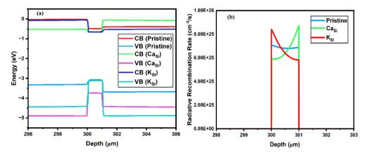
Fig. 18 (a) Energy band diagram of the proposed LED utilizing pristine SiC,  $K_{Si}$ , and  $Ca_{Si}$  as an active layer at an applied bias of 5 V; (b) radiative recombination characteristics of the proposed LED utilizing pristine SiC,  $K_{Si}$ , and  $Ca_{Si}$  as an active layer.
