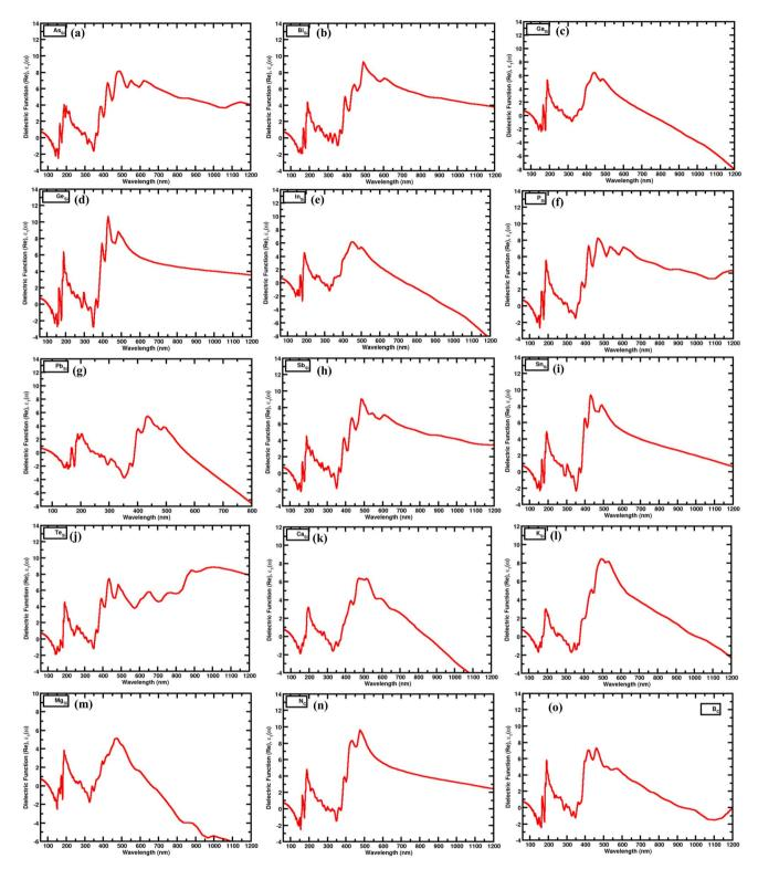
Fig. 8 The real part of the dielectric spectrum of point doping in a monolayer of SiC: (a)  $As_{Si}$ , (b)  $Bi_{Si}$ , (c)  $Ga_{Si}$ , (d)  $Ge_{Si}$ , (e)  $In_{Si}$ , (f)  $P_{Si}$ , (g)  $Pb_{Si}$ , (h)  $Sb_{Si}$ , (i)  $Sn_{Si}$ , (j)  $Te_{Si}$ , (k)  $Ca_{Si}$ , (l)  $K_{Si}$ , (m)  $Mg_{Si}$ , (n)  $N_{C}$ , (o)  $B_{C}$ .
