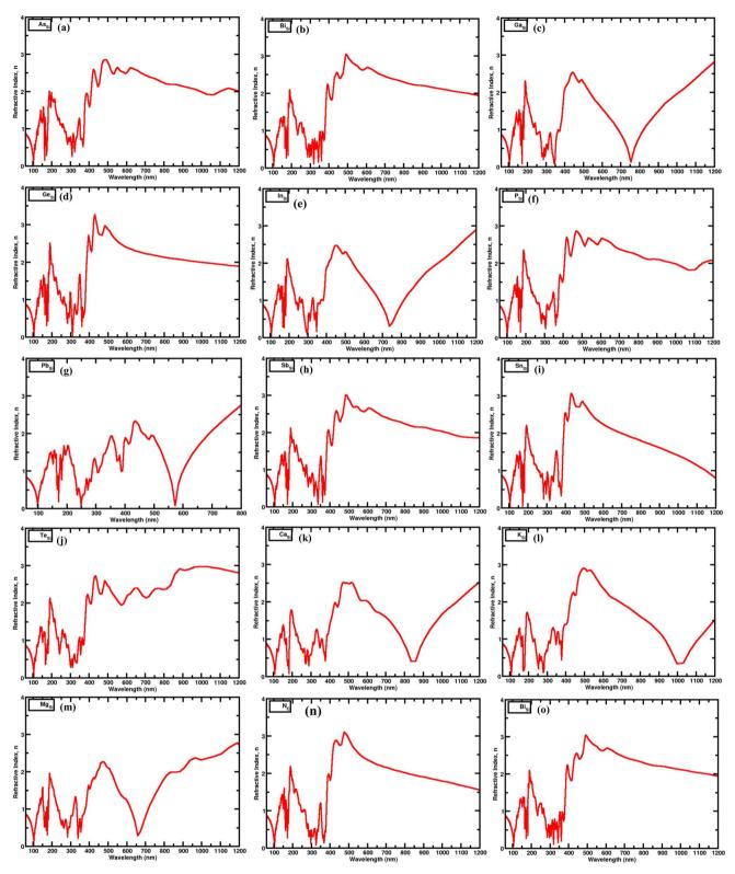
Fig. 12 The refractive index of point doping in a monolayer of SiC: (a)  $As_{Si}$ , (b)  $Bi_{Si'}$ , (c)  $Ga_{Si'}$ , (d)  $Ge_{Si'}$ , (e)  $In_{Si'}$ , (f)  $P_{Si'}$ , (h)  $Sh_{Si'}$ , (i)  $Sn_{Si'}$ , (j)  $Te_{Si'}$ , (k)  $Ca_{Si}$ , (I)  $K_{Si}$ , (m)  $Mg_{Si}$ , (n)  $N_C$ , (o)  $B_C$ .
