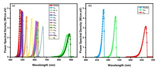
Fig. 17 (a) Power spectrum density as a function of wavelength for SiC-based LED; (b) the peak of the power spectral density is seen at 480 nm, 534 nm, and 668 nm, respectively. Here, the power spectrum density, which stands for the optical power emitted per unit area per unit energy interval, is represented in W cm $^{-1}$  eV $^{-1}$ .
