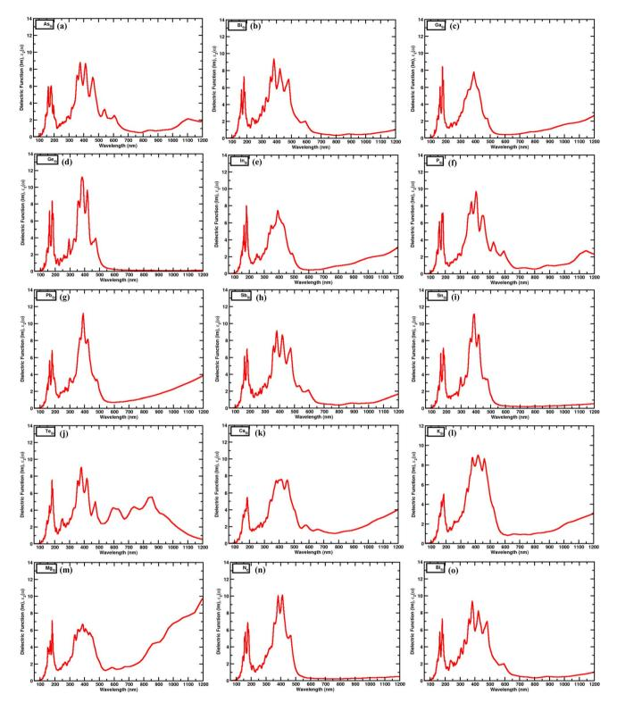
Fig. 10 The imaginary part of the dielectric spectrum of point doping in a monolayer of SiC: (a)  $As_{Si}$ , (b)  $Bi_{Si}$ , (c)  $Ga_{Si}$ , (d)  $Ge_{Si}$ , (e)  $In_{Si}$ , (f)  $P_{Si}$ , (g)  $Pb_{Si}$ , (h)  $Sb_{Si}$ , (i)  $Sn_{Si}$ , (j)  $Te_{Si}$ , (k)  $Ca_{Si}$ , (l)  $K_{Si}$ , (m)  $Mg_{Si}$ , (n)  $N_{C}$ , (o)  $B_{C}$ .
