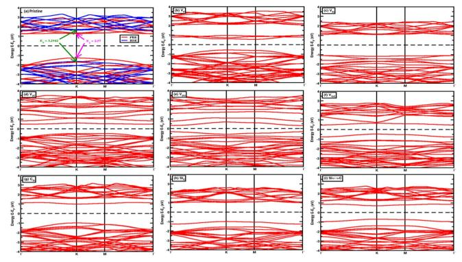
Fig. 5 (a) The electrical band diagrams of a pristine 2D-SiC monolayer; the electrical band diagrams of single vacancy defect in a monolayer of SiC: (b)  $V_{C}$ , (c)  $V_{Si}$ ; the electrical band diagrams of double vacancy defect in a monolayer of SiC: (d)  $V_{2C}$ , (e)  $V_{2Si}$ , (f)  $V_{SiC}$ ; the electrical band diagrams of antisite defect in a monolayer of SiC: (g)  $C_{Si}$ , (h) Si<sub>C</sub>, (i) Si  $\leftrightarrow$  C.
