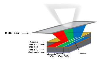
Fig. 21 A white LED device is a composite of red, green, and blue integrated LED chips, where  $W_{\rm R}$  and  $W_{\rm G}$  represent the width of the K<sub>Si</sub> and Ca<sub>Si</sub>, respectively, and  $W_{\rm B}$  represents the width of the pristine 2D SiC as an active layer. Dielectric trenches (e.g., SiO<sub>2</sub>) provide lateral isolation. Each zone has a separate transparent top contact (e.g., ITO), with a shared N-type bottom contact.
