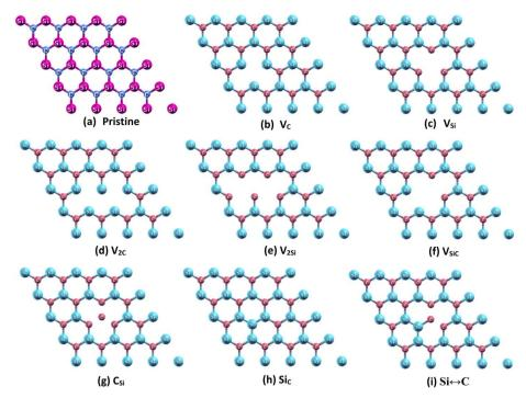
Fig. 1 (a) The structural configuration of pristine monolayer SiC; the structural configuration of single vacancy defect in a monolayer of SiC: (b)  $V_{C_r}$  (c)  $V_{S_i}$ ; the structural configuration of double vacancy defect in a monolayer of SiC: (d)  $V_{2C_r}$  (e)  $V_{2S_i}$  (f)  $V_{SiC}$ ; the structural configuration of antisite defect in a monolayer of SiC: (g)  $C_{Si_r}$  (h)  $Si_{C_r}$  (i) Si  $\leftrightarrow$  C.
