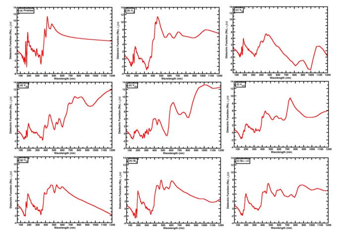
(a) The real part of the dielectric spectrum of a pristine 2D-SiC monolayer; the real part of the dielectric spectrum of single vacancy defect in a monolayer of SiC: (b)  $V_C$ , (c)  $V_{Si}$ ; the real part of the dielectric spectrum of double vacancy defect in a monolayer of SiC: (d)  $V_{2C}$ , (e)  $V_{2Si}$ , (f)  $V_{SiC}$ ; the real part of the dielectric spectrum of antisite defect in a monolayer of SiC: (g)  $C_{Si}$ , (h)  $Si_{C}$ , (i)  $Si \leftrightarrow C$ .
