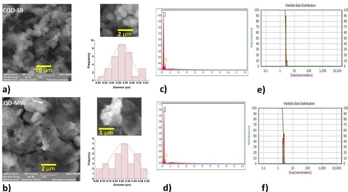
Fig. 1 (a) and (b) SEM images of micro-sized colloidal CDs in CQD-SB and CQD-MW, along with the histograms representing the frequency of the observed particle diameters in  $\mu\text{m}$ , overlaid with fitted Gaussian curves to illustrate distribution symmetry and spread; (c) and (d) EDX pattern of CQDs showing C and O as main elements; (e) and (f) DLS data showing particle size distribution.
