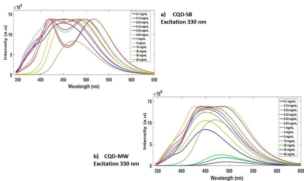
Fig. 6 Photoluminescence emission spectra of CQDs at 330 nm. (a) CQD-SB at varying concentrations ( $0.1\text{--}40\text{ mg mL}^{-1}$ ). (b) CQD-MW at varying concentrations ( $0.1\text{--}40\text{ mg mL}^{-1}$ ); both CQDs indicate distinct emissive states, followed by spectral broadening and reduced intensity at higher concentrations.
