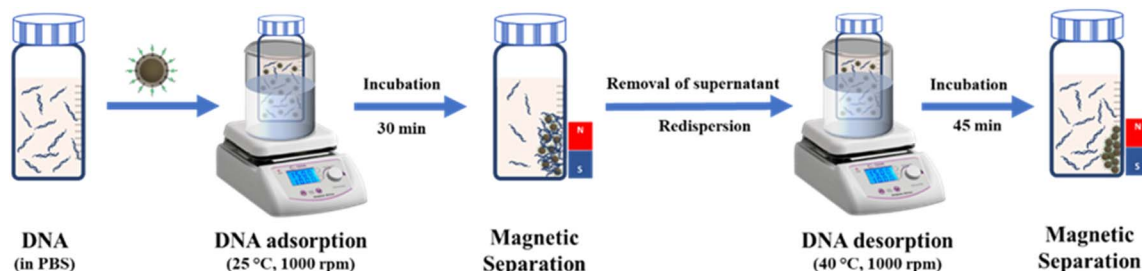
Scheme 4 Schematic illustration of the adsorption and desorption procedure of DNA using functionalized/modified iron oxide magnetic nanoparticles.
