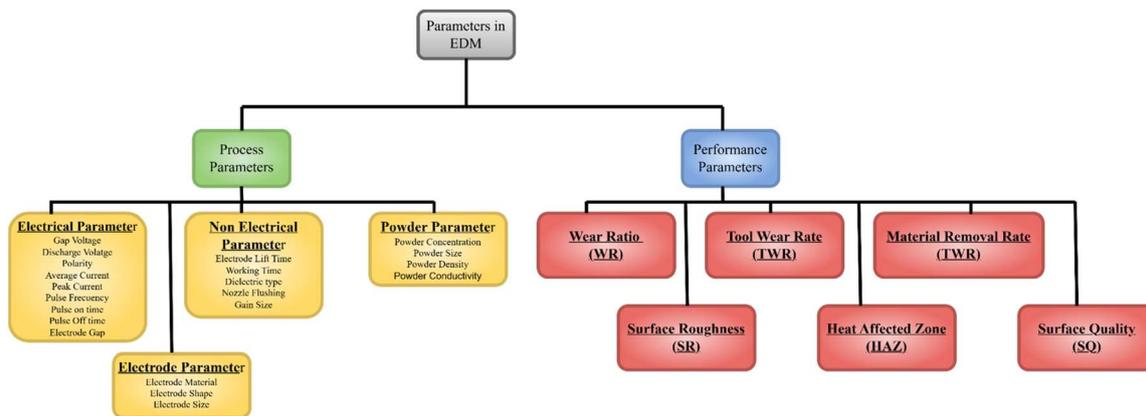
Fig. 17 Several process parameters affecting machining of SMAs.<sup>427</sup>
