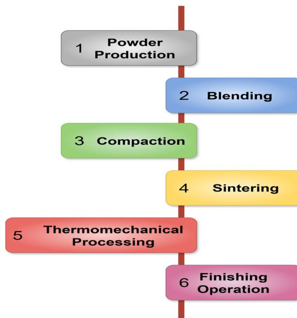
Fig. 15 Steps of powder metallurgy.<sup>337</sup>
