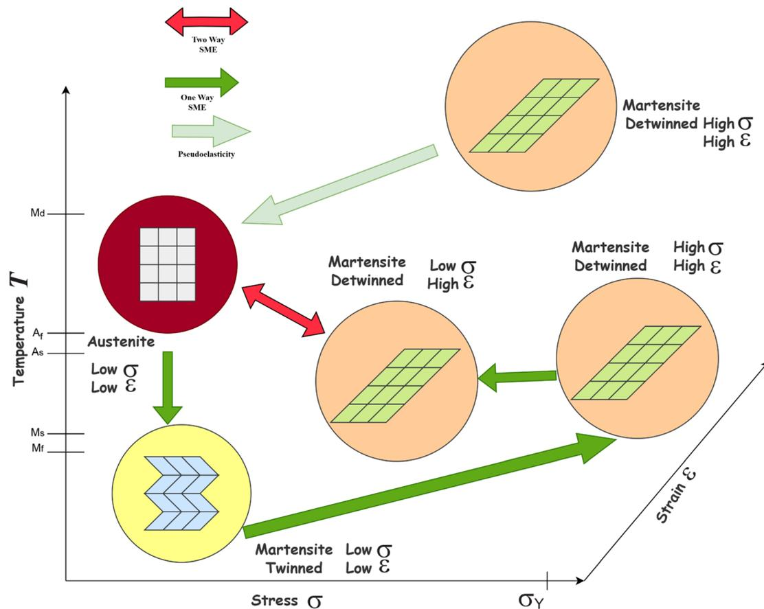
Fig. 3 Phase transformation behaviour of SMA.<sup>17</sup>
