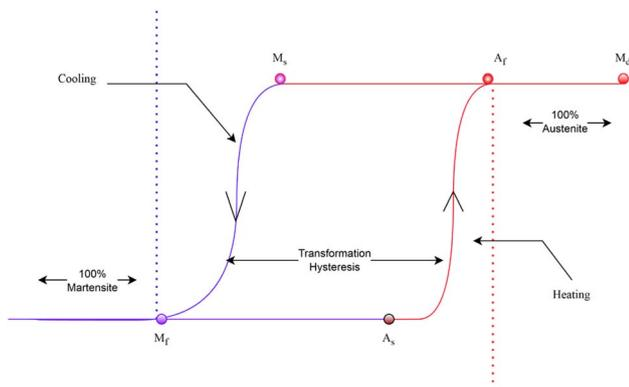
Fig. 4 Transformation temperatures in a phase transformation cycle.<sup>36</sup>
