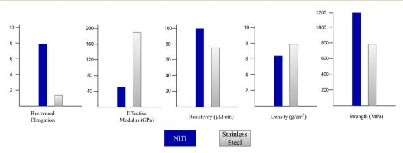
Fig. 11 Comparison of some properties between NiTi and SS.<sup>76</sup>
