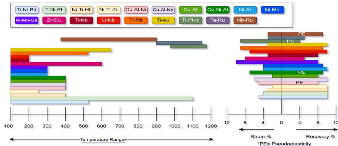
Fig. 7 Temperature range of some HTSMAs with their pseudoelasticity.<sup>17</sup>
