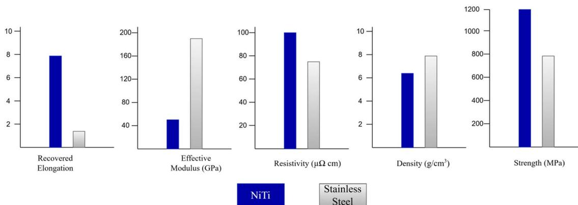
Fig. 11 Comparison of some properties between NiTi and SS.<sup>76</sup>
