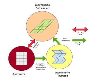
Fig. 2 Two crystal structures of SMA and their transformation relationship.
