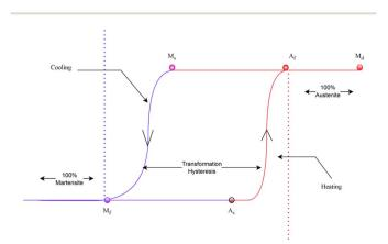
Fig. 4 Transformation temperatures in a phase transformation cycle.<sup>36</sup>
