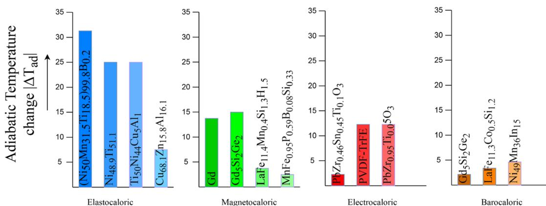
Fig. 6 Comparison of cooling effect of some caloric materials.<sup>45</sup>
