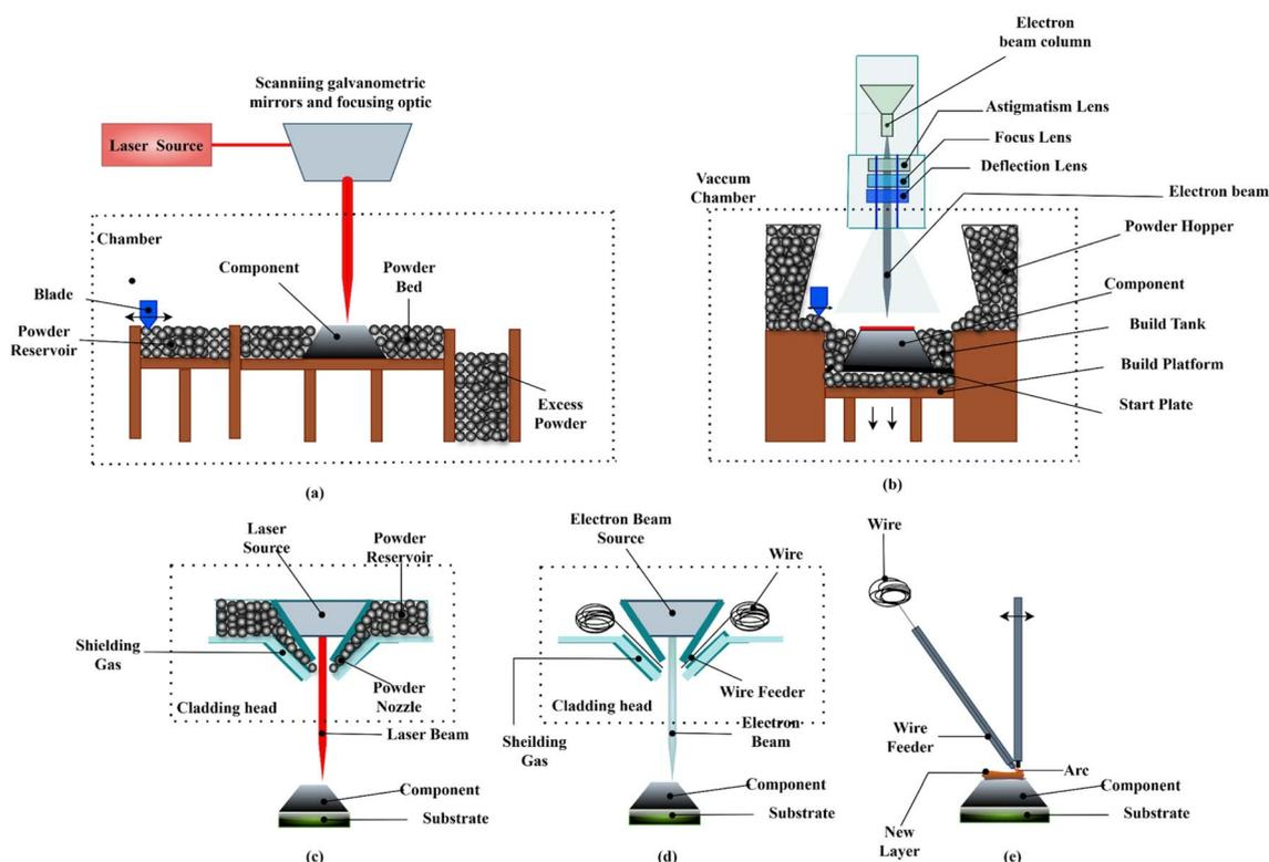
Fig. 16 Schematic of additive manufacturing processes (a) PBF-L (b) PBF-EB (c) DED-L (d) DED-EB (e) DED-Arc.<sup>392</sup>
