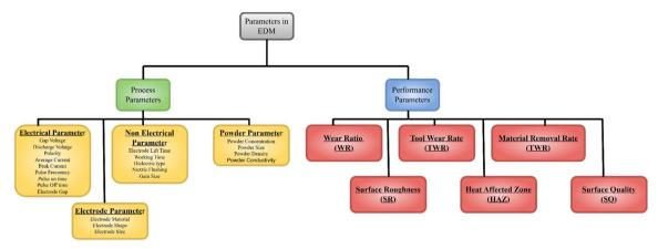
Several process parameters affecting machining of SMAs. 427
