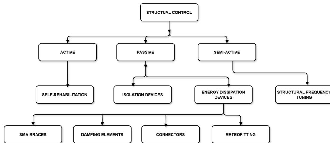
Fig. 12 SMA-based structural control systems.<sup>125</sup>
