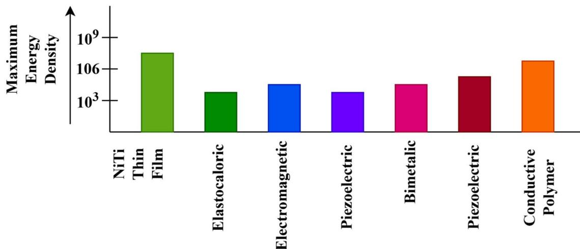
Fig. 8 Superior energy density of NiTi thin film.<sup>17</sup>
