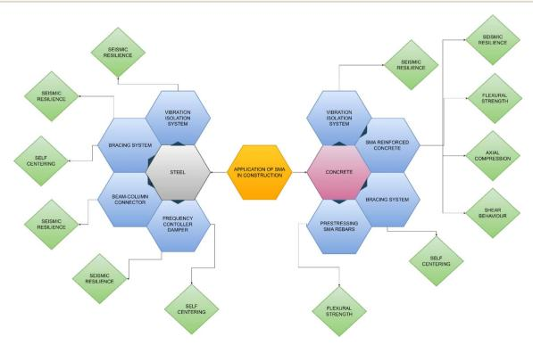
Fig. 13 SMA-based systems in construction engineering
