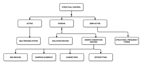
Fig. 12 SMA-based structural control systems. 125
