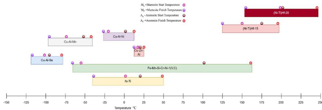
Fig. 5 Working temperature ranges of different SMAs.<sup>17</sup>
