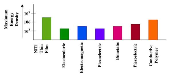
Fig. 8 Superior energy density of NiTi thin film.<sup>17</sup>
