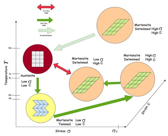
Fig. 3 Phase transformation behaviour of SMA.17
