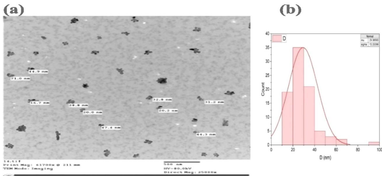
Fig. 6 (a) TEM micrograph of synthesized REO NPs and (b) their particle size distribution histogram.
