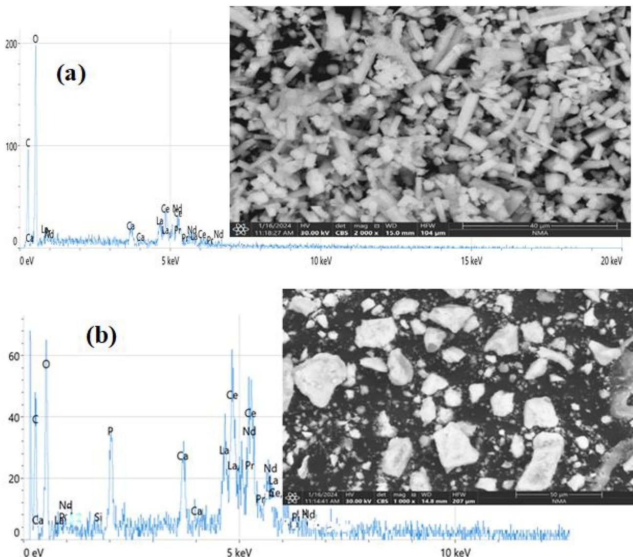
Fig. 5 SEM image and EDS spectra of (a) REO cake and (b) REO NPs.
