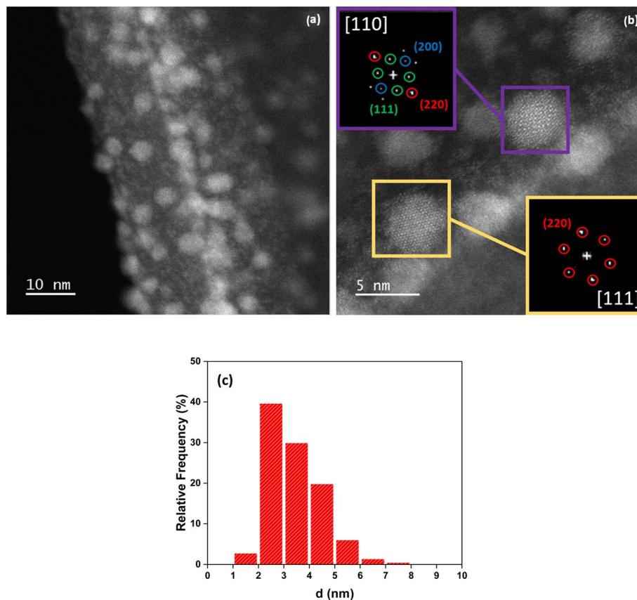
Fig. 7 STEM-HAADF images of Sn NPs dispersed in ethylene glycol after the reaction of SnCl<sub>2</sub> with AA at 80 °C for 16 h. (a) Low resolution and (b) high resolution images of two Sn NPs in [110] and [111] zone axes with their indexed FFT. (c) Particle diameter histogram.
