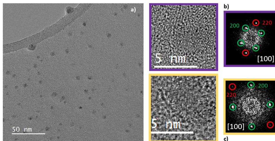
Fig. 4 (a) HRTEM image of the Cu NPs synthesized in EG and 0.4 mL HCl (35%) after  $\text{H}_2$  treatment at  $300^\circ\text{C}$  for 1 hour. (b and c) HRTEM images of two representative Cu NPs in the [001] zone axis with their indexed FFT.
