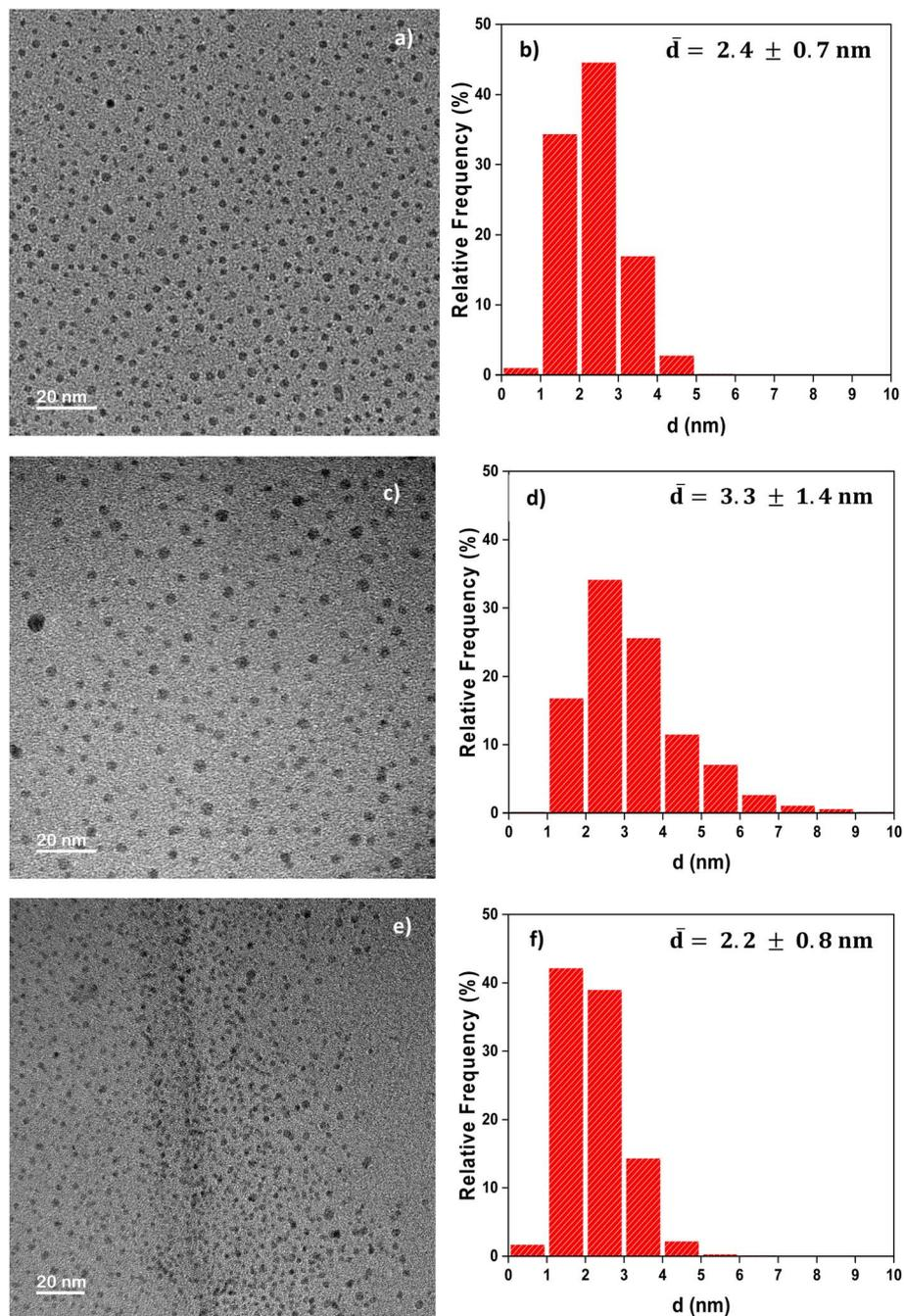
Fig. 2 TEM images and particle diameter histograms of Cu NPs obtained from the reduction of  $\text{CuCl}_2$  by AA in various solvents at  $80^\circ\text{C}$  for 16 h: (a and b) ethylene glycol, (c and d) ethylene glycol with the addition of 0.4 mL of HCl (35%) and (e and f) diethylene glycol.
