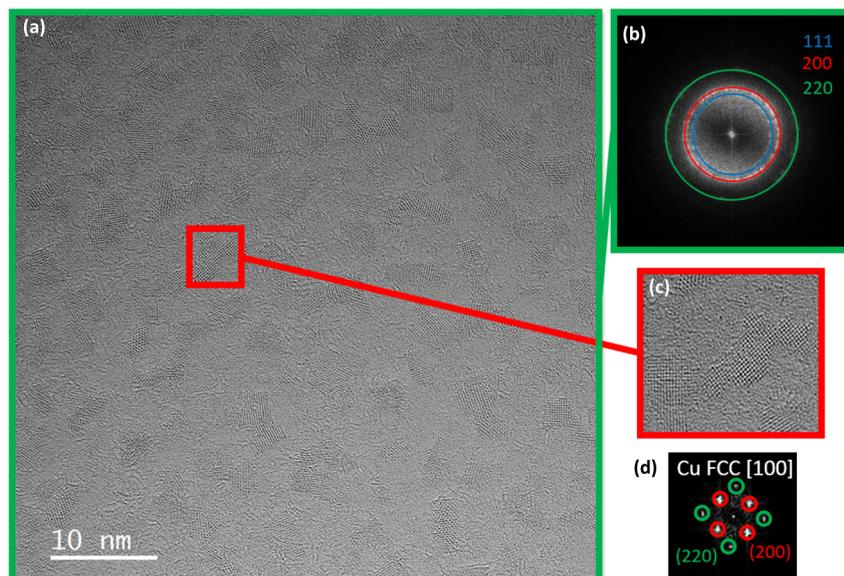
Fig. 5 (a) HRTEM image of Cu NPs synthesized in DEG. (b) Reduced Fourier transform of the whole area showing the three families of planes with lower indices for FCC structures: (200) (red), (111) (blue) and (220) (green). (c) HRTEM image of a specific area of (a) containing a NP. (d) Reduced Fourier transform of the NP in (b) matching with FCC Cu in the [100] direction.
