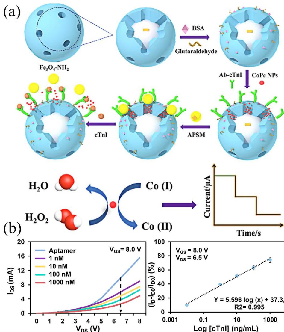
Fig. 7 (a) The preparation process of the APASM-capped CoPc NPs  $\text{Fe}_3\text{O}_4\text{-Ab/MGCE}$  sandwich electrochemical immunosensor; reproduced from ref. 133 with permission from Elsevier, copyright 2019. (b) Molecular recognition of cTnI at concentrations from  $1.0 \text{ ng mL}^{-1}$  to  $1.0 \text{ } \mu\text{g mL}^{-1}$  using an Au/PCN-FET biosensor and corresponding calibration curve. Reproduced from ref. 134 with permission from MDPI, copyright 2022.
