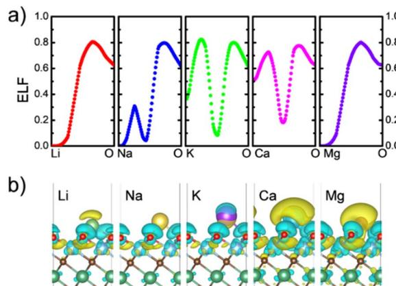
Fig. 6 (a) ELF line profiles along the O-ion bond. (b) Charge density difference isosurfaces with an isovalue of 0.002 e Å<sup>-3</sup>; yellow and aqua colors represent charge accumulation and depletion, respectively.
