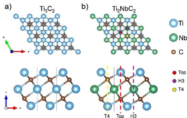
Fig. 1 Top and side views of (a) Ti<sub>3</sub>C<sub>2</sub> MXene and (b) Ti<sub>2</sub>NbC<sub>2</sub> MXene.
