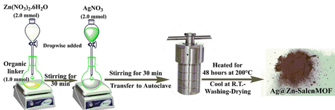
Scheme 1 Proposed two-step hydrothermal synthesis mechanism of the \text{Ag@Zn-SalenMOF} composite. Step 1: formation of a \text{Zn}(\text{II}) -organic linker adduct (solution 1) via coordination of \text{Zn}(\text{NO}_3)_2 \cdot 6\text{H}_2\text{O} with the salen-based nano-linker. Step 2: incorporation of Ag nanoparticles through DMF-mediated reduction of \text{AgNO}_3 , followed by hydrothermal treatment ( 200^\circ\text{C} , 8 hours) to assemble the hierarchical \text{Ag@Zn-SalenMOF} structure. The composite is obtained as a light green-brown precipitate with 81.3% yield and thermal stability exceeding 300^\circ\text{C} .
