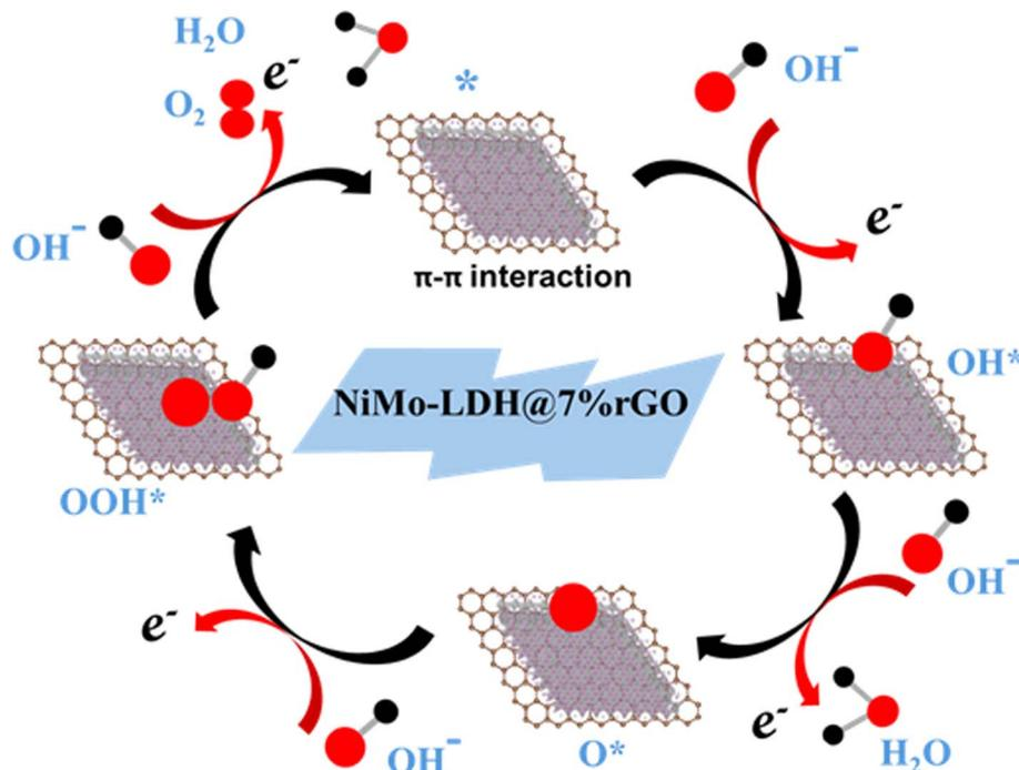
Fig. 6 Proposed mechanism of the OER on the surface of NiMo-LDH@7% rGO.
