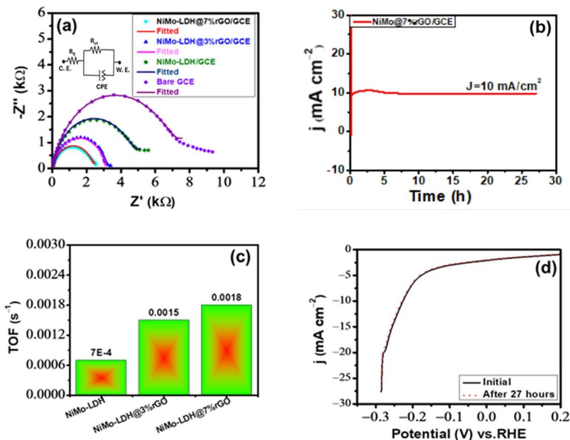
Fig. 11 (a) Electrochemical impedance spectra recorded in 0.5 M H<sub>2</sub>SO<sub>4</sub> solution, with corresponding Randel's circuit as shown in the inset. (b) Chronoamperometry test up to 27 hours. (c) TOF calculation for HER. (d) LSV performed before and after 27 hour chronoamperometric test.
