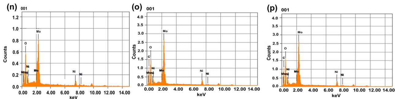
Fig. 3 FE-SEM images of (a–c) NiMo–LDH at 500 nm, 300 nm, 2  $\mu\text{m}$  (d–f) NiMo–LDH@3%rGO at magnifications of 500 nm, 300 nm, 2  $\mu\text{m}$  (g–i) NiMo–LDH@7%rGO 500 nm, 300 nm 2  $\mu\text{m}$ . (j–m) Elemental mapping of Ni, Mo, C, O. (n–p) EDX spectra of NiMo–LDH, NiMo–LDH@3%rGO and NiMo–LDH@7%rGO respectively.
