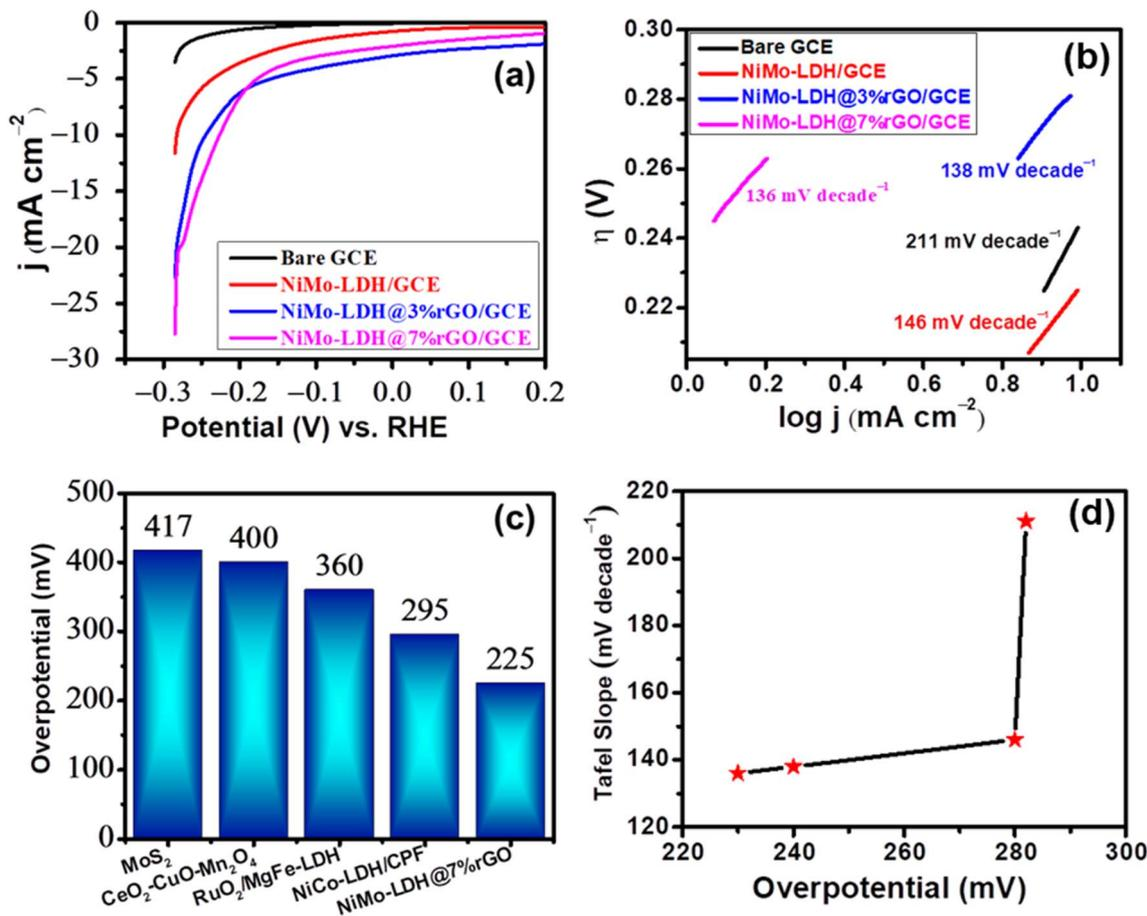
Fig. 10 (a) LSV curves obtained at bare GCE, NiMo-LDH/GCE, NiMo@3% rGO/GCE, and NiMo-LDH@7% rGO/GCE in 0.5 M H<sub>2</sub>SO<sub>4</sub>. (b) Tafel slope analysis for the synthesized electrocatalysts in acidic medium. (c) Comparison of NiMo-LDH@7% rGO/GCE with reported HER electrocatalysts. (d) Relationship between Tafel slope and overpotential.
