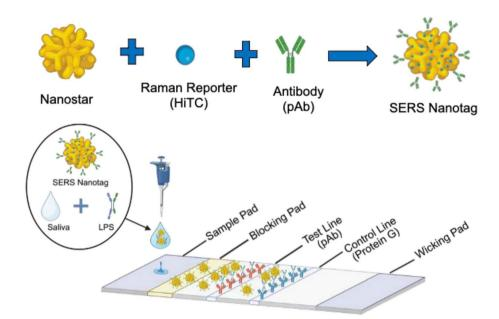
Fig. 1 Basic operation of the antibody sandwich LFA using the SERS Nanotag (created in BioRender).
