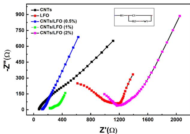
Fig. 11 Electrochemical impedance spectroscopy (EIS) spectra (Nyquist plots) of CNTs, LFO, and CNTs/LFO nanocomposites, showing imaginary impedance ( $-Z''$ ) versus real impedance ( $Z'$ ). Measurements were performed at an open-circuit potential with a 10 mV AC amplitude over the frequency range 10 000–0.1 Hz. The spectra were fitted to an equivalent circuit model to extract key parameters such as charge transfer resistance ( $R_{ct}$ ).
