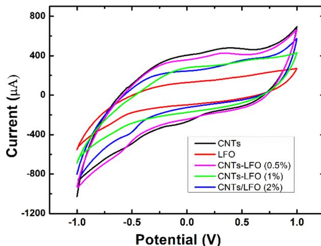
Fig. 8 Cyclic voltammetry (CV) responses of SPEs modified with CNTs, lithium ferrite (LFO), and CNTs/LFO nanocomposites. Measurements were recorded in 5 mM [Fe(CN)<sub>6</sub>]<sup>3-/4-</sup> (1 : 1) containing 0.1 M KCl by scanning the potential from  $-1.0$  to  $+1.0$  V at a scan rate of 50 mV s<sup>-1</sup>.
