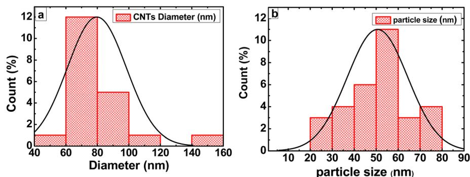
Fig. 6 Histograms of the diameter and particle size distributions for (a) CNTs and (b) lithium ferrite (LFO).
