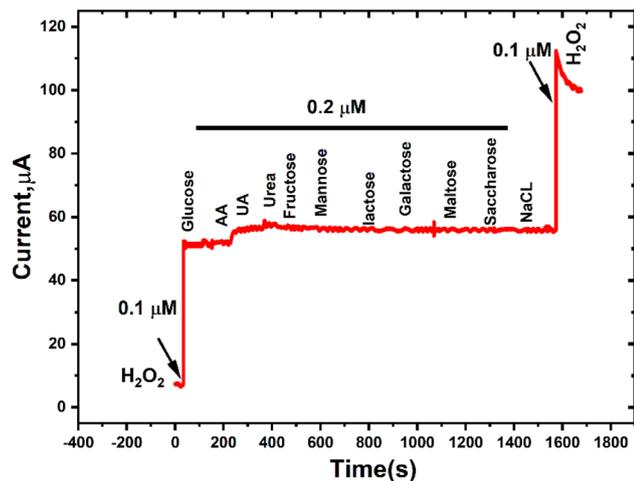
Fig. 16 Chronoamperometric responses of the CNTs/LFO-modified electrode to sequential additions of 0.1  $\mu\text{M}$   $\text{H}_2\text{O}_2$  and 0.2  $\mu\text{M}$  of common potential interferents, including ascorbic acid (AA), uric acid (UA), urea, fructose, mannose, lactose, maltose, sucrose, NaCl, and glucose.
