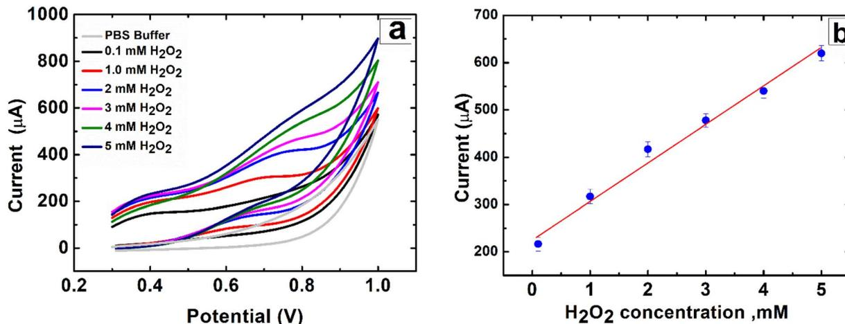
Fig. 12 (a) Cyclic voltammograms recorded for CNTs/LFO-modified SPEs in the presence of varying H<sub>2</sub>O<sub>2</sub> concentrations, using phosphate-buffered saline (PBS, pH = 7.4) as the supporting electrolyte. (b) Corresponding calibration curve of the current response versus H<sub>2</sub>O<sub>2</sub> concentration, demonstrating the electrocatalytic performance of the CNTs/LFO electrode.
