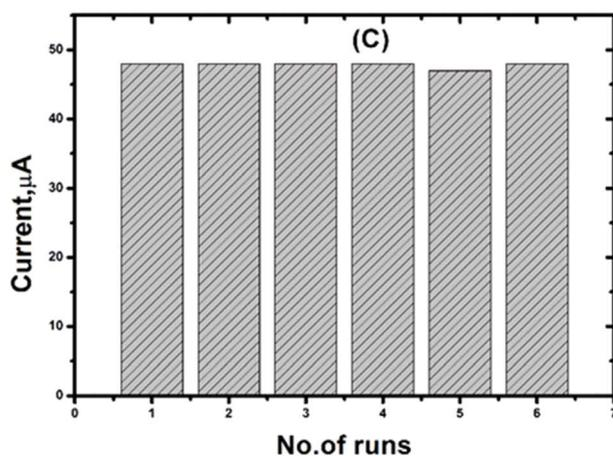
Fig. 17 (A) Stability of the CNTs/LFO-modified electrode toward 0.1  $\mu\text{M}$   $\text{H}_2\text{O}_2$ . (B) Reproducibility of the sensor response using six independently prepared electrodes. (C) Repeatability of the electrode fabrication process under identical conditions. All measurements were conducted using sequential injections of 0.1  $\mu\text{M}$   $\text{H}_2\text{O}_2$ .
