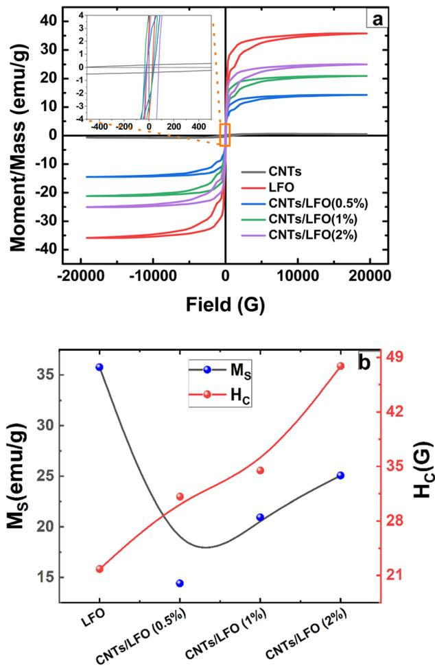
Fig. 7 Magnetic measurements obtained using vibrating sample magnetometry (VSM): (a) hysteresis loops of pure CNTs and CNTs/LiFe<sub>5</sub>O<sub>8</sub> nanocomposites recorded at room temperature over an applied magnetic field range of  $\pm 20$  kG, and (b) comparison of the saturation magnetization and coercivity values of CNTs/LiFe<sub>5</sub>O<sub>8</sub> nanocomposites with those of pristine lithium ferrite.
