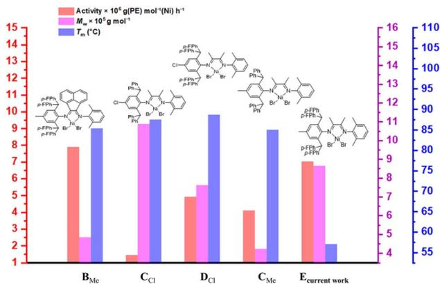
Fig. 7 A comparative analysis of the catalytic performance among a series of  $\alpha$ -diimine nickel complexes, featuring either the 1,2-bis(arylimino)acenaphthene or the 2,3-bis(arylimino)butane ligand backbone, was conducted under identical polymerization conditions (Al/Ni ratios of 2000 : 1, 30 °C, 30 min, 10 atm).
