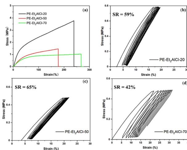
Fig. 10 (a) Stress-strain curves and (b–d) recovery tests for the selected polyethylene samples, PE-Et<sub>2</sub>AlCl-20, PE-Et<sub>2</sub>AlCl-50, and PE-Et<sub>2</sub>AlCl-70.
