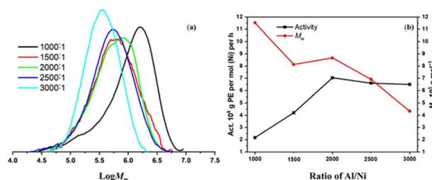
Fig. 2 (a) GPC traces and (b) plots of catalytic activity and M<sub>w</sub> of the polyethylene produced using Ni1/MAO at different Al/Ni molar ratios (entries 1–5, Table 2).
