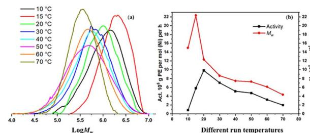
Fig. 3 (a) GPC traces and (b) plots of catalytic activity and M<sub>w</sub> of the polyethylene produced using Ni1/MAO at different run temperatures (entries 8, 6–12, Table 2).
