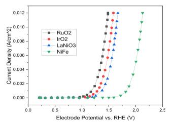
Fig. 7 Polarization curve for RuO<sub>2</sub>, IrO<sub>2</sub>, LaNiO<sub>3</sub>, Ni-Fe at 25C.
