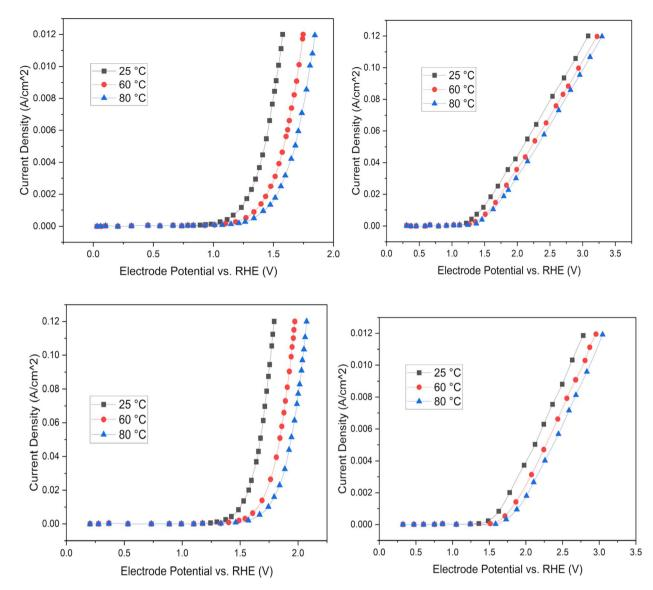
Fig. 6 Polarization curve for RuO<sub>2</sub>, IrO<sub>2</sub>, LaNiO<sub>3</sub>, Ni-Fe at different temperatures.
