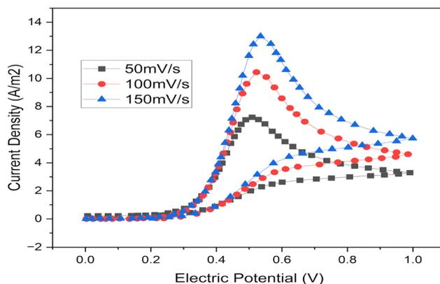
Fig. 4 Cyclic voltammogram of Ni–Fe at 50 mV s<sup>-1</sup>, 100 mV s<sup>-1</sup>, 150 mV s<sup>-1</sup>.
