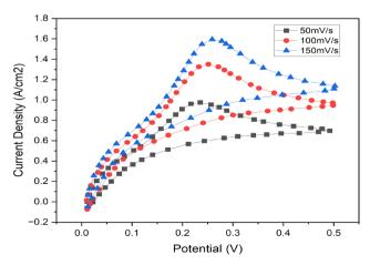
Fig. 3 Cyclic voltammogram of IrO<sub>2</sub> at 50 mV s<sup>-1</sup>, 100 mV s<sup>-1</sup>, 150 mV  $_{\rm c}^{-1}$
