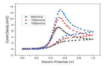
Fig. 4 Cyclic voltammogram of Ni–Fe at 50 mV  $\rm s^{-1},\ 100\ mV\ s^{-1},\ 150\ mV\ s^{-1}.$
