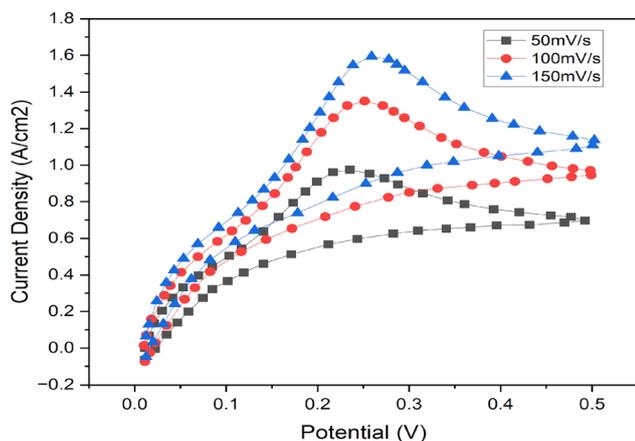
Fig. 3 Cyclic voltammogram of IrO<sub>2</sub> at 50 mV s<sup>-1</sup>, 100 mV s<sup>-1</sup>, 150 mV s<sup>-1</sup>.
