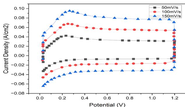
Fig. 2 Cyclic voltammogram of RuO<sub>2</sub> at 50 mV s<sup>-1</sup>, 100 mV s<sup>-1</sup>, 150 mV s<sup>-1</sup>.
