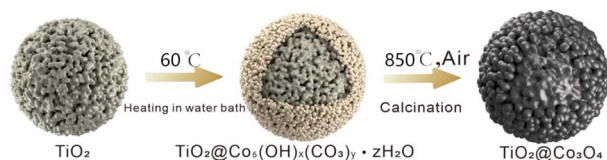
Fig. 1 Schematic diagram of preparation of \text{TiO}_2@Co_3O_4 microspheres.
