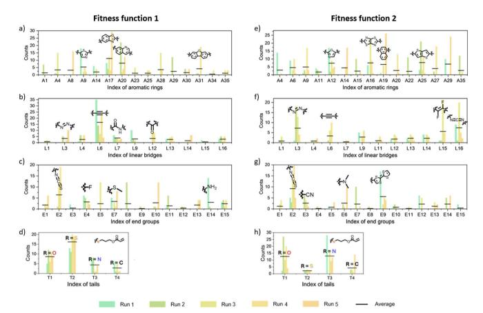
Fig. 7 Building block frequencies of each of five genetic algorithm runs with Fitness functions 1 and 2, including (a and e) aromatic rings, (b and f) linear bridges, (c and g) end groups, (d and h) tails.
