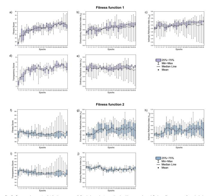
Fig. 5 Score and property distributions across all five independent genetic algorithm runs: (a and f) show fitness score, (b and g) show extraordinary refractive index  $n_{\text{ev}}$ , (c and h) show average refractive index  $n_{\text{avg}}$ , (d and i) show transparency score, (e and j) show ordinary refractive index  $n_{\text{o}}$  for Fitness functions 1 and 2, respectively.
