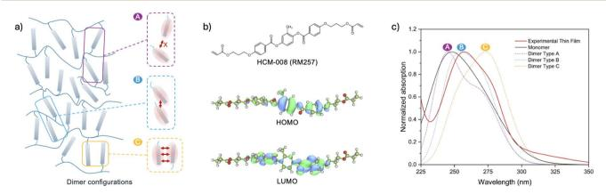
Fig. 2 (a) Schematic illustration of a liquid crystal polymer network featuring three distinct dimer conformations, each representing varying degrees of  $\pi$ - $\pi$  stacking interactions. (b) Structure of HCM-008 and its HOMO-LUMO orbitals. (c) UV absorption spectra of HCM-008 from experimental monomer solution, polymer thin film and computational results of different dimer types.
