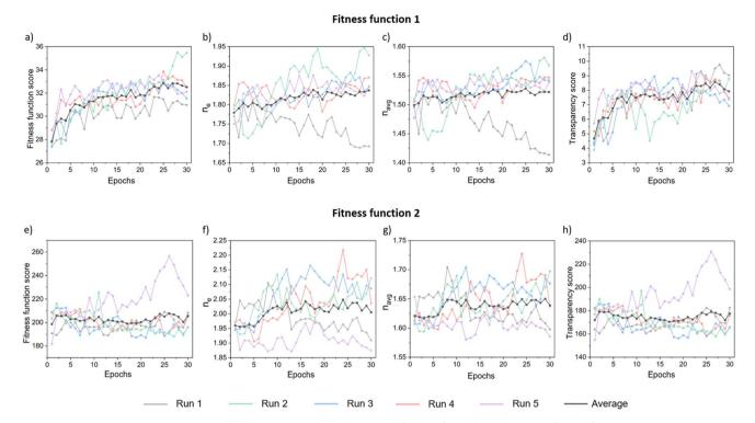
Fig. 6 Metrics across each of the five independent genetic algorithm runs: (a and e) show fitness score, (b and f) show extraordinary refractive index  $n_{e}$ , (c and g) show average refractive index  $n_{avq}$ , (d and h) show transparency score for Fitness functions 1 and 2, respectively.
