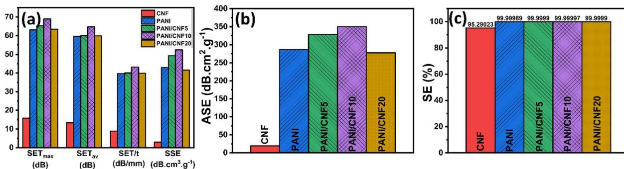
Fig. 2 Shielding performance of CNF, PANI, PANI/CNF5, PANI/CNF10 and PANI/CNF20 in the K-band frequency region (18 GHz to 26.5 GHz) in terms of (a) SE<sub>max</sub>, SET<sub>av</sub>, SET/*t* and SSE (b) ASE (c) SE (%).
