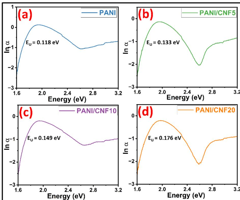
Fig. 5 Plot of  $\ln \alpha$  vs. energy of (a) PANI, (b) PANI/CNF5, (c) PANI/CNF10 and (d) PANI/CNF20.
