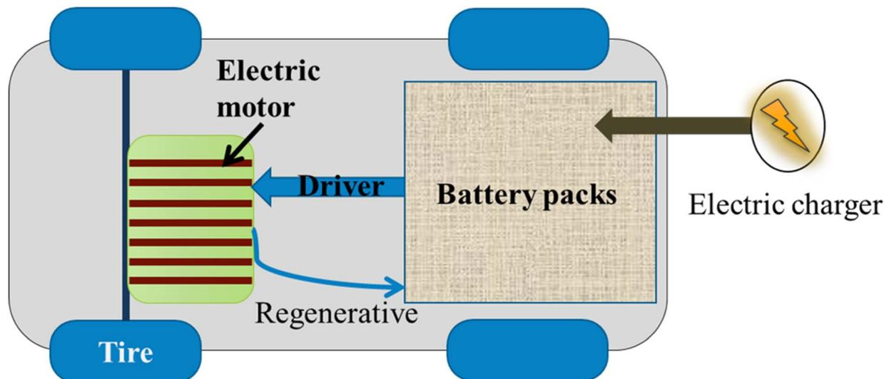
Fig. 6 Main components of battery electric vehicles.
