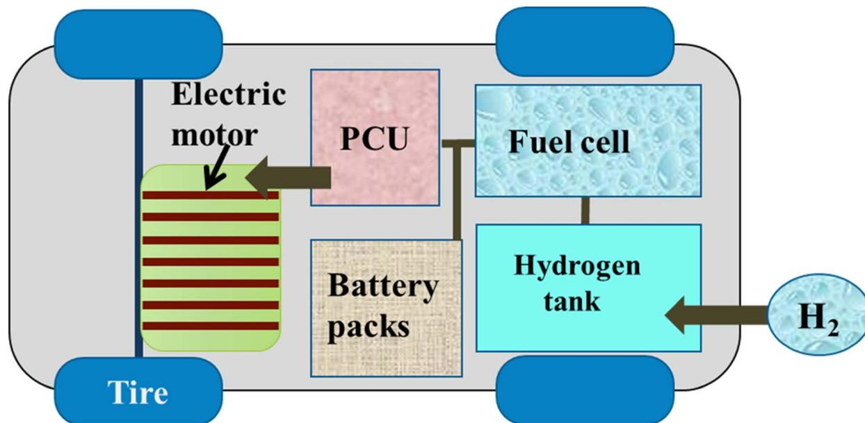
Fig. 9 Main components of fuel cell electric vehicles.
