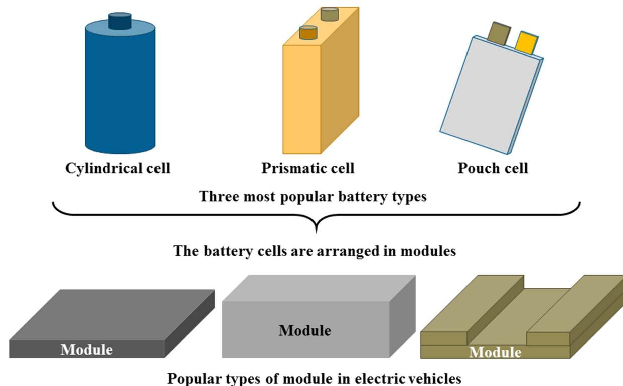
Fig. 3 The three most popular electric vehicle battery modules are based on three different cell types.
