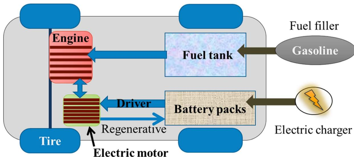
Fig. 8 Main components of plug-in hybrid electric vehicles.
