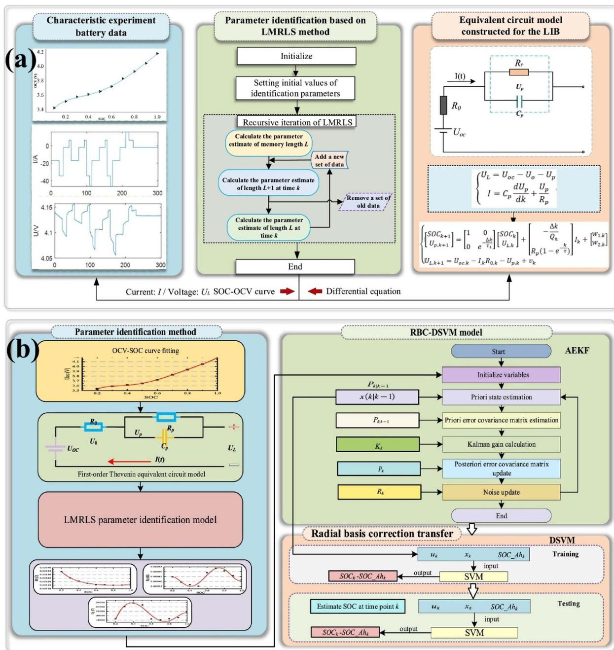
Fig. 17 Flowchart of (a) adaptive online parameter identification method and (b) RBC-DSVM model. Figure adapted from Wang *et al.*<sup>199</sup> Copyright 2024 Elsevier.
