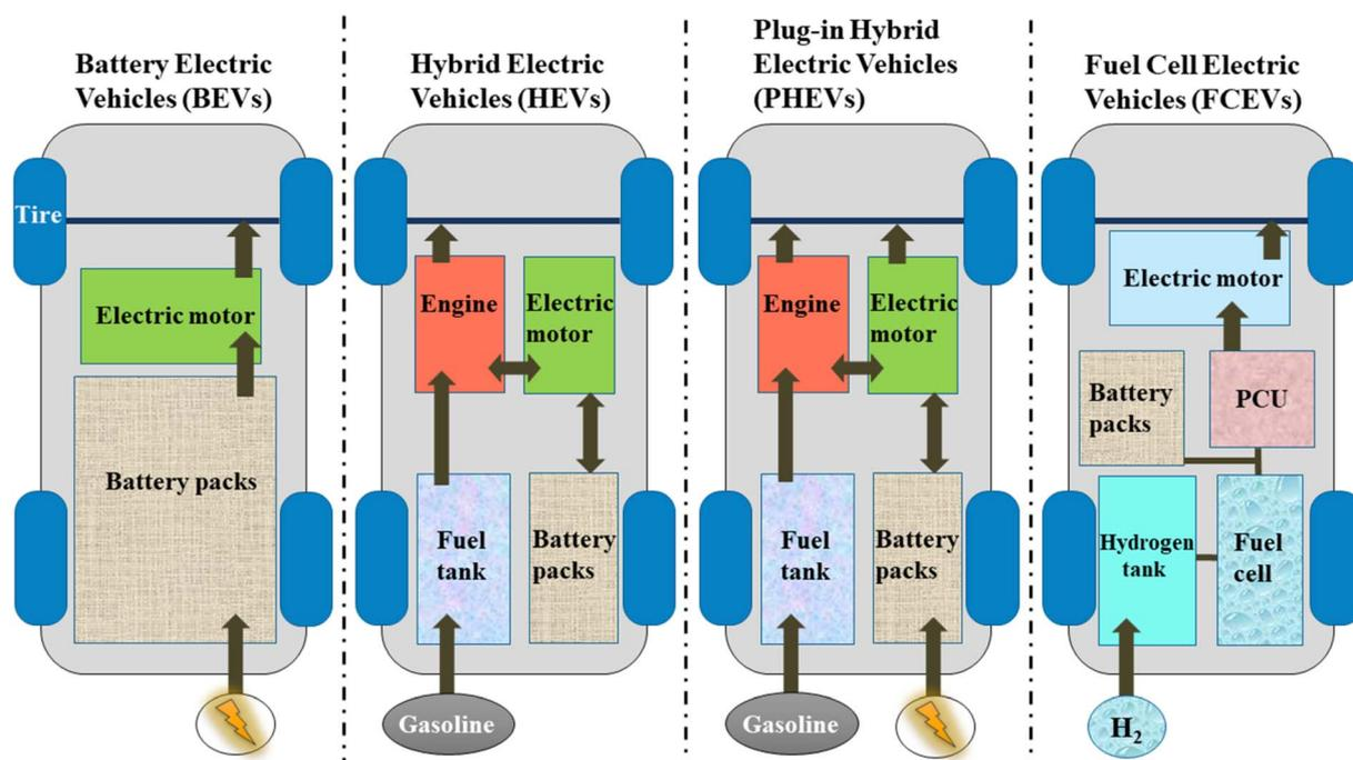
Fig. 5 The general construction of four most popular electric vehicles.
