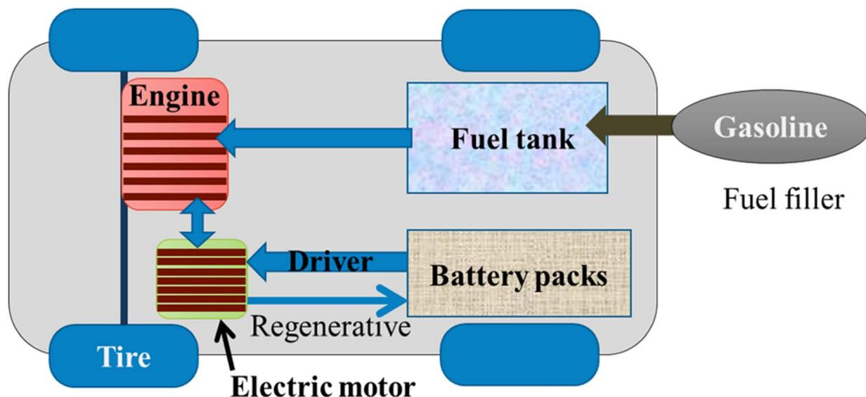
Fig. 7 Main components of hybrid electric vehicles.
