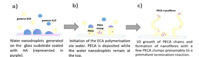
Fig. 5 Illustration of the 1D growth of PECA-NF *via* the DAGS mechanism which was unveiled when using HA as a ‘tracing agent’: (a) the water nanodroplets are formed on the surface coated with HA (purple dots); (b) the polymerisation of ECA is initiated by water and eventually, by a few HA molecules. The water insoluble PECA is deposited. The water nanodroplets with solubilised HA remain on the top; (c) 1D growth of the PECA macromolecules and formation of PECA-NF.
