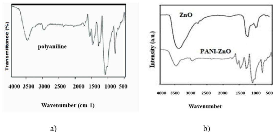
Fig. 2 FT-IR spectra of (a) polyaniiline and (b) ZnO and PANI-ZnO.
