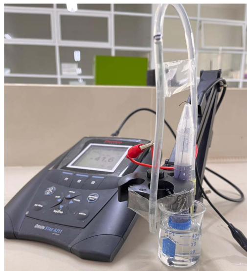
Fig. 1 Fabricated electrodes in a potentiometer.
