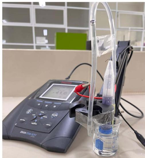
Fig. 1 Fabricated electrodes in a potentiometer.
