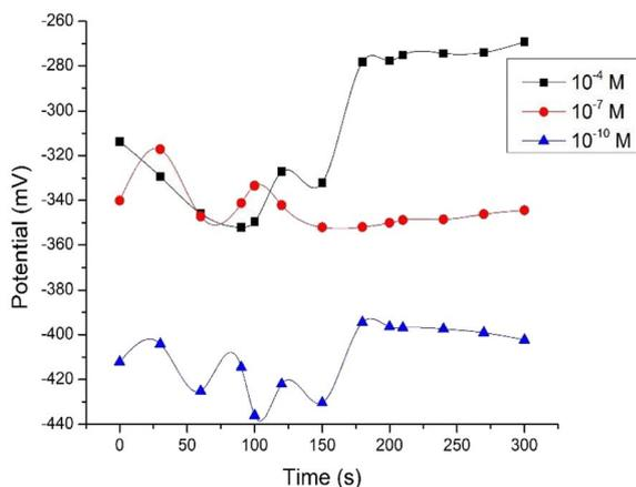
Fig. 6  $\text{Al}^{3+}$  ISE response time curve.
