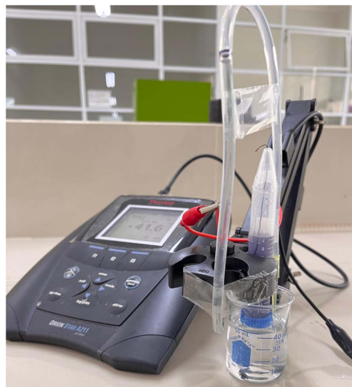
Fig. 1 Fabricated electrodes in a potentiometer.
