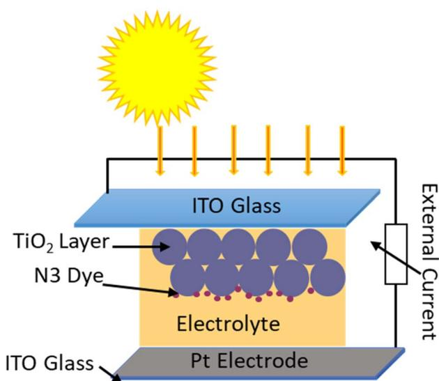
Fig. 1 Schematic diagram of DSSC fabrication.
