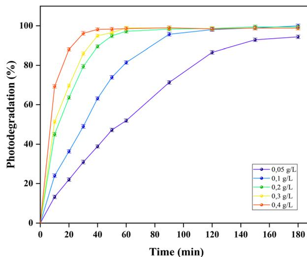
Fig. 8 Effect of catalyst amount on percentage degradation of CFX (CFX conc. 10 ppm, free pH).
