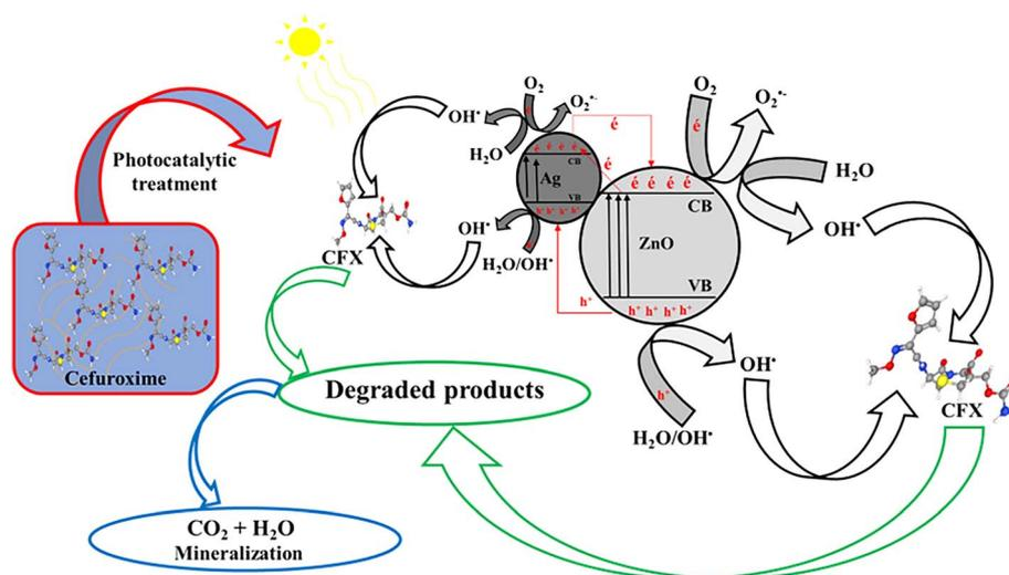
Fig. 15 Plausible photocatalytic degradation mechanism of CFX.
