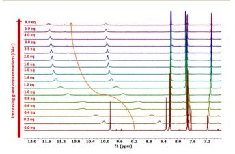
Fig. 9  $^{1}$ HNMR titration spectra (600 MHz, DMSO- $d_{6}$ ) measured upon incremental addition of the guest TBAOAc (0  $\rightarrow$  8 eq) to a BUR-2 (2 mM) at 298 K.
