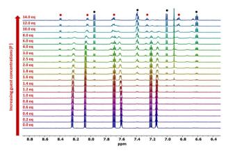
Fig. 5 Expanded <sup>1</sup>HNMR chemical shifts (600 MHz, DMSO- $d_6$ ) of aromatic protons (H's) measured upon incremental addition of the guest TBAF (0  $\rightarrow$  14 eq) to a solution of BUR-1 (2 mM) at 298 K. <sup>1</sup>H NMR Signals correspond to 1,3-dihydro-2H-benzimidazol-2-one ( $\blacksquare$ ) and to o-nitroaniline ( $\blacksquare$ ).
