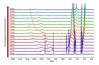
Fig. 6  $^{1}$ HNMR titration spectra (600 MHz, DMSO- $d_{6}$ ) upon incremental addition of the guest TBAF (0  $\rightarrow$  14 eq) to a solution of BUR-2 (2 mM) at 298 K.
