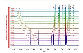
Fig. 8  $\,^{1}$ HNMR titration spectra (600 MHz, DMSO- $d_{6}$ ) measured upon incremental addition of the guest TBAOAc (0  $\rightarrow$  8 eq) to a solution of BUR-1 (2 mM) at 298 K.  $^{1}$ H NMR Signals correspond to 1,3-dihydro-2H-benzimidazol-2-one ( $\bullet$ ) and to o-nitroaniline ( $\bullet$ ).
