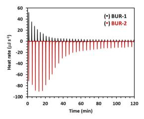
Fig. 3 Overlaid ITC raw heats for sequential injection of the fluorine anion ( $F^-$ ) solution to 2.0 mM solutions of receptor BUR-1 and BUR-2 in DMF at 25 °C.
